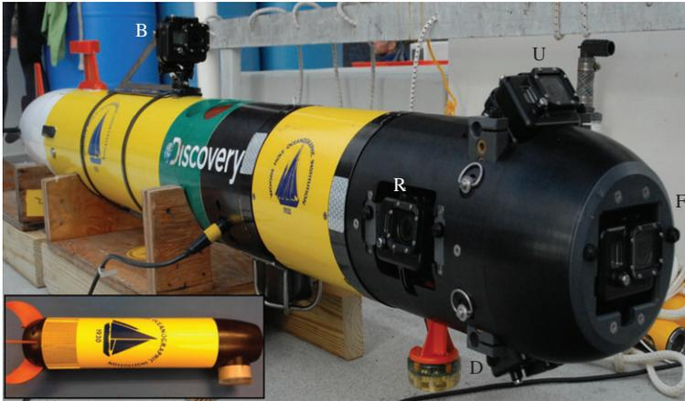
FIG. 2. Autonomous underwater vehicle and transponder (inset) used to track *Carcharodon carcharias* off the coast of Guadalupe Island, Mexico. Video cameras mounted in nose were oriented directly forward (F), upward (U), downward (D), right (R) and left (L, not shown). The backward facing camera (B) was mounted topside for tracks WS01, WS02 and WS03, and on the underside for the three tracks of WS04.
