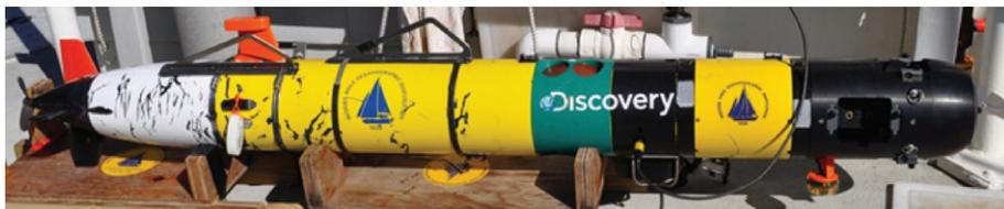
FIG. 9. Autonomous underwater vehicle with tooth rakes resulting from nine bites from *Carcharodon carcharias*; note that all of the marks are located on the lower aft section of the vehicle.
