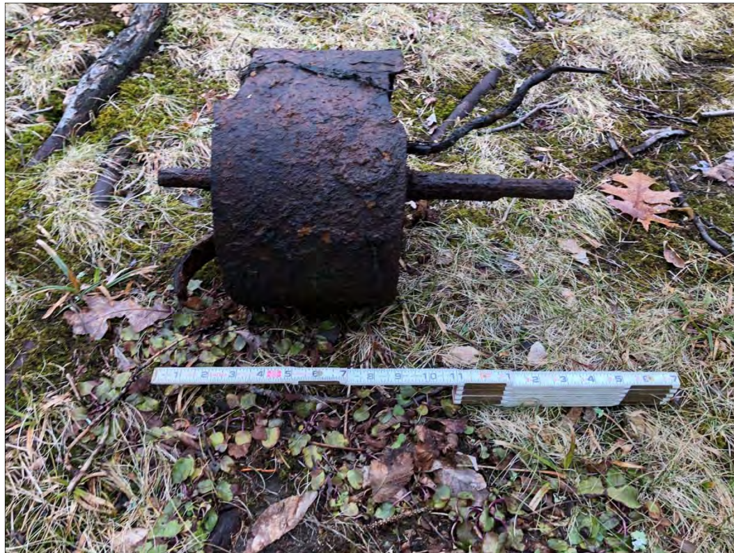
Figure 38. Iron pulley with line shaft found in western wheel pit of mill foundation: a) interior assembly view; and b) exterior lengthwise view with shaft at both ends.
