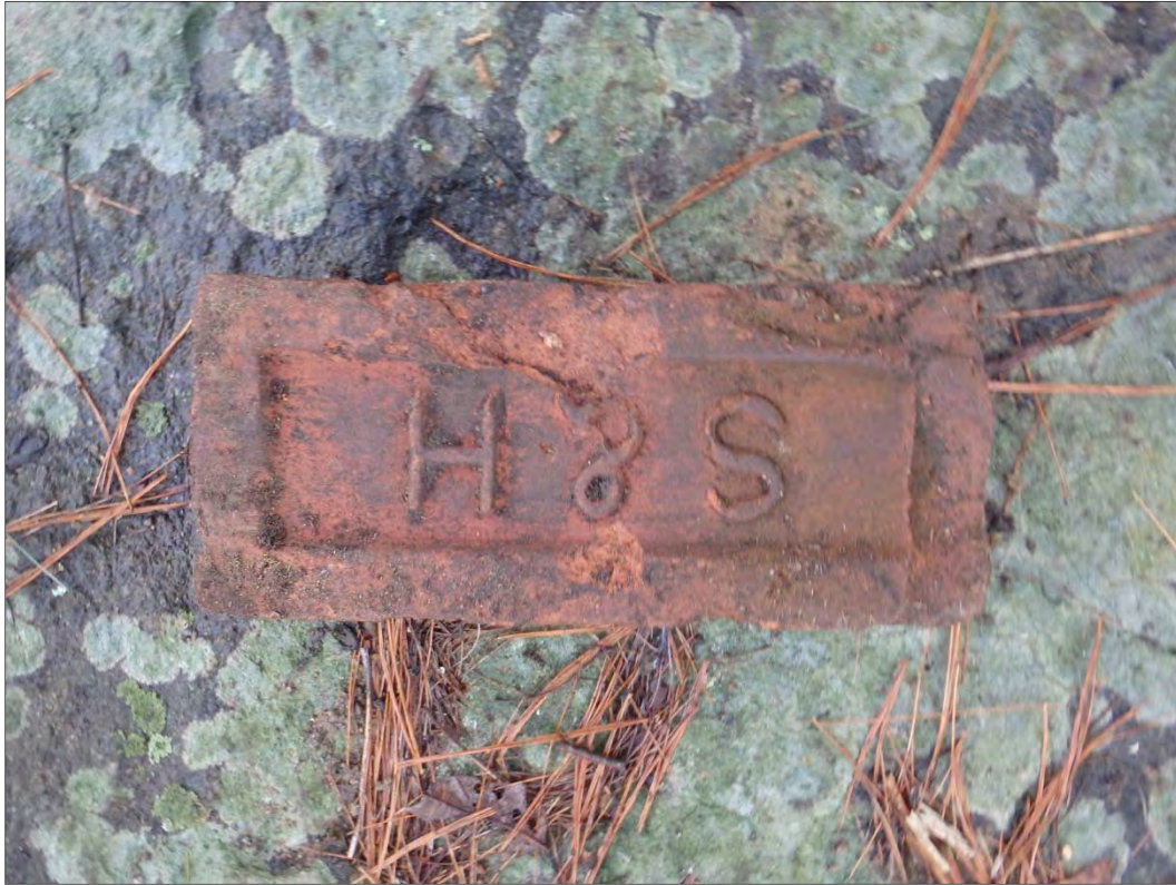
Figure 46. “S & H” stamped brick noted in earthen dam fill.
