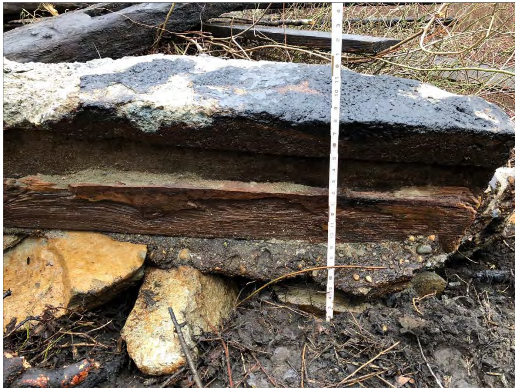
Figure 37. Concrete slab with embedded timber removed from across river bottom in east channel (spillway).
