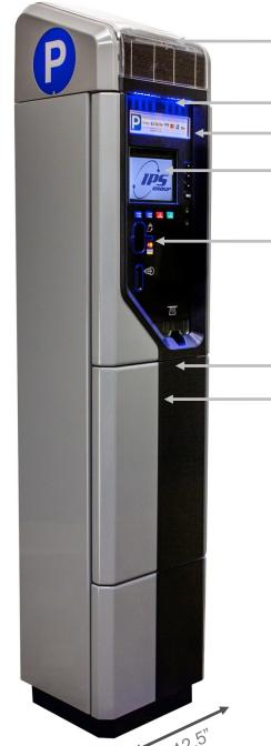
solar panel LED lighting 4G modem armored glass screen credit card reader stainless steel housing secured coin vault Available in pay-by-space, pay and display, and pay-by-plate ADA Compliant, max button height 48", screen height 45" PA-DSS & PCI-DSS Certified
