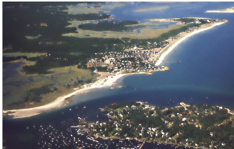
Photograph 1.13. Barrier beach system. The two spits stemming off of the developed section are barrier beaches. Most of the heavily developed section is not considered barrier beach because it lies seaward of an upland, not a wetland or waterbody.
