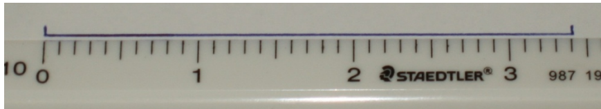
Photograph F3. Using an engineer scale. Where a plan indicates the scale is 1"=10', this line measures 34 feet using the engineer scale (the line measured 3.4 and 3.4 \times 10 = 34 feet).
