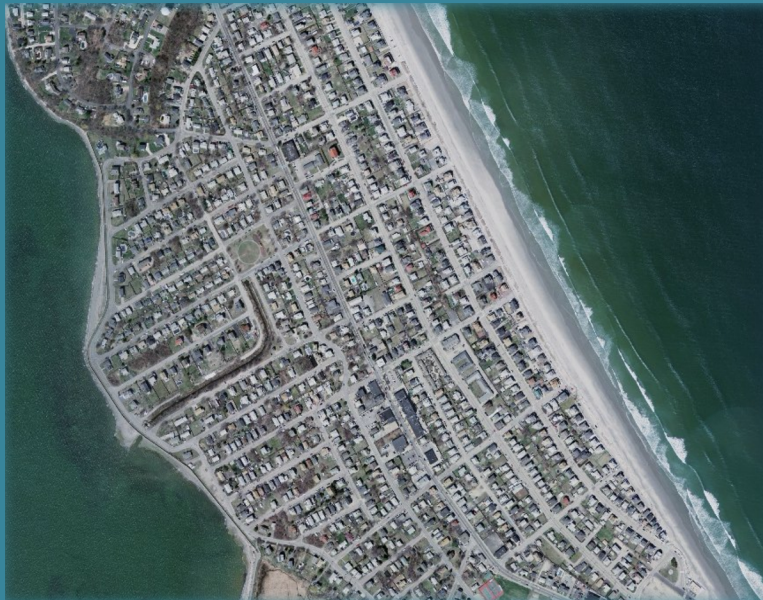
Photograph 4.3. Barrier beach that has lost much of its ability to function. Photograph courtesy of the Office of Geographic Information (MassGIS) and United States Geological Survey (USGS) Color Ortho Imagery 2008 30cm.
