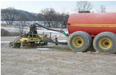
Figure 2: Complete one pass spreader system with aeration attachment
