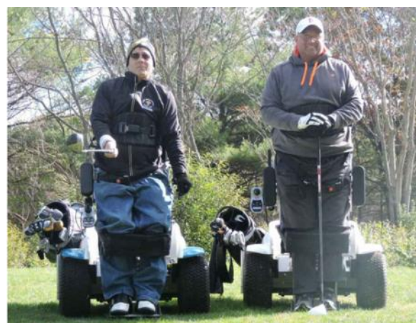
ParaGolfers are all-terrain wheelchairs that assist golfers into a standing position to swing.
