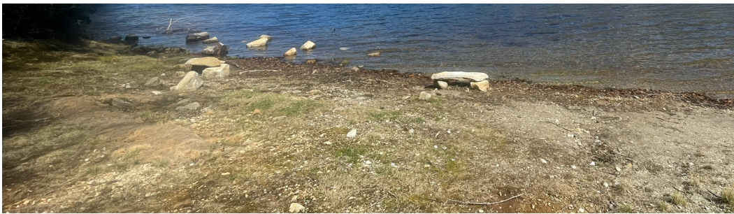
Image 4. Bioswales will replace a vegetated area, pictured here, along the slope between the parking lot and the beach. This will help slow the flow of stormwater runoff and decrease beach scouring and erosion.
