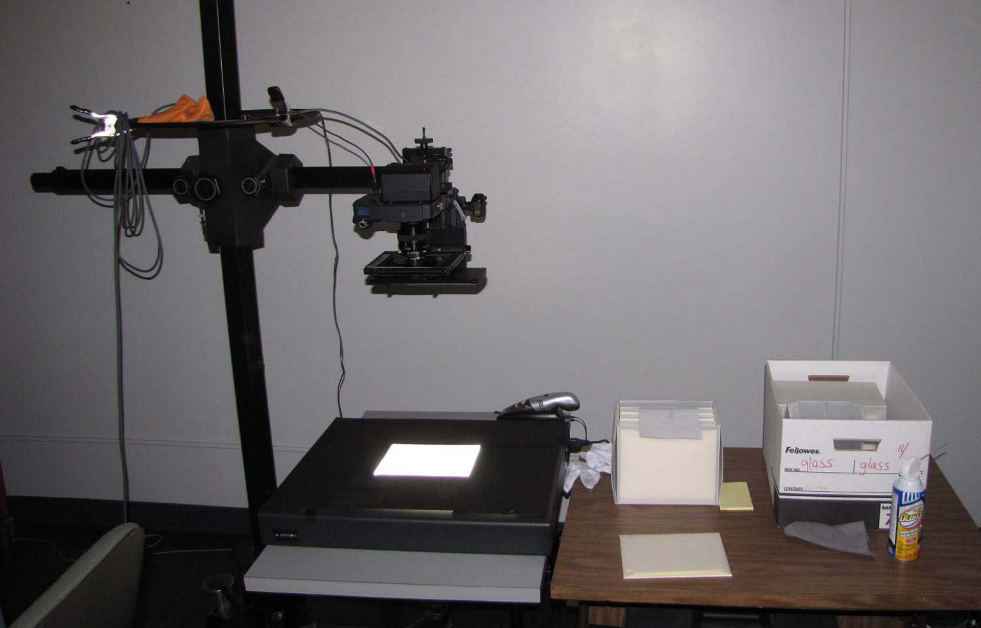
BPL's digitizing the MWW glass plate negatives using a light table and digital camera
