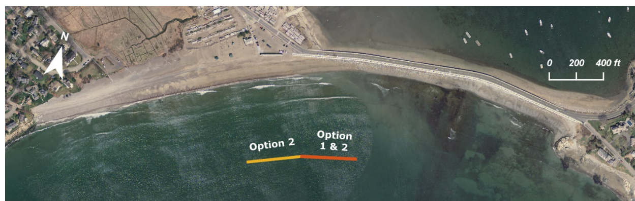
Figure 2-20. Position of modeled Devereux Beach reef options. Both reef sections have a crest elevation of +4 ft MLW and are 400 feet long.
