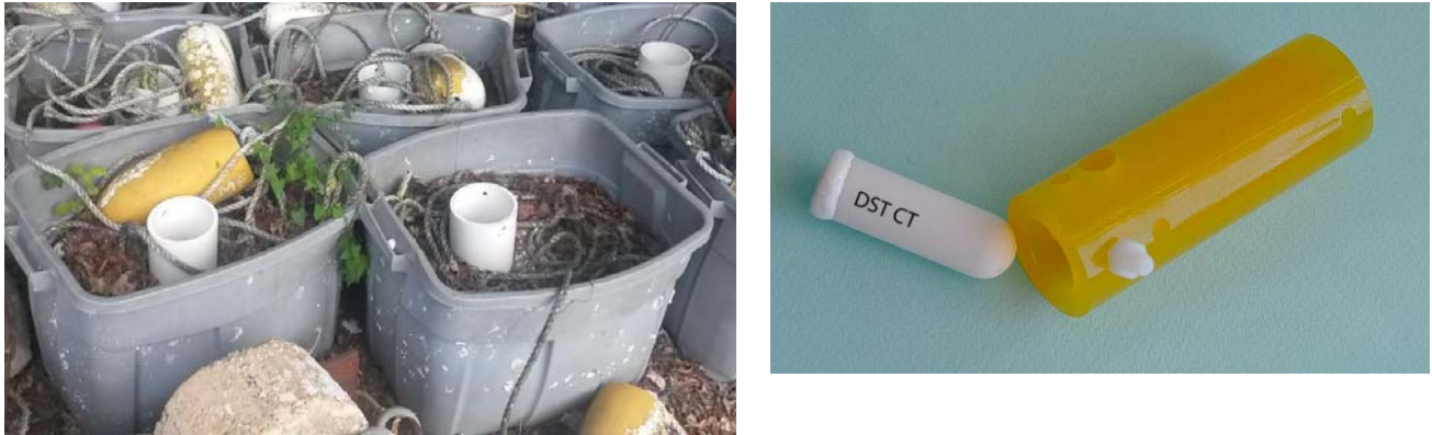
Figure 1D-12. Image of the (a) cement tub mooring system and (b) the plastic sleeve that housed the Starr-Oddi DST depth logger.
