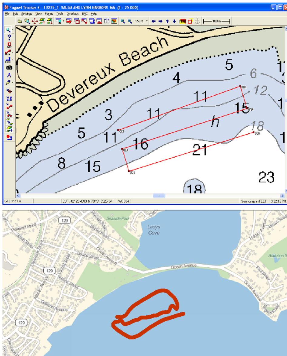
Figure 1D-15. Planned and realized track lines for spatial surface water sampling. The velocity of the vessel was c. 2 kt (1 m/s).
