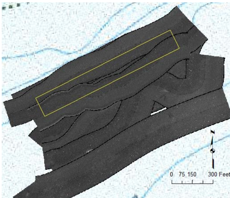
Figure 1D-4. Sidescan sonar mosaic at Long Island (Gallops control site). Yellow box identifies target study area.
