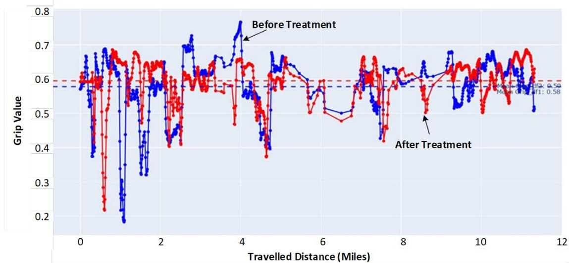
**Figure 3-4: Grip values before and after treatment for the manual mode**
