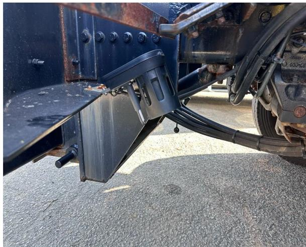
**Figure 2-4: Current MD30 sensor installed on the MassDOT truck**
