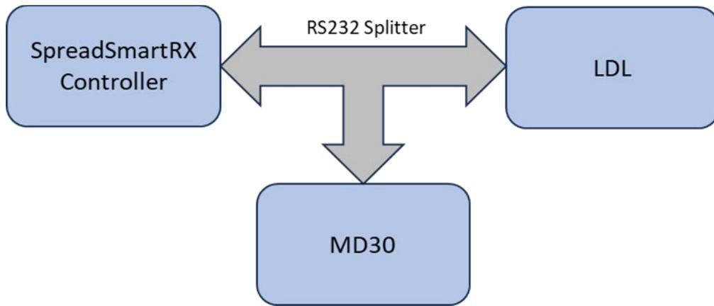
**Figure 6-10: Y splitter connection**
