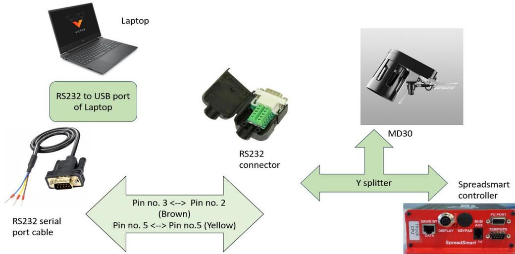
**Figure 6-12: Connection setup block diagram**
