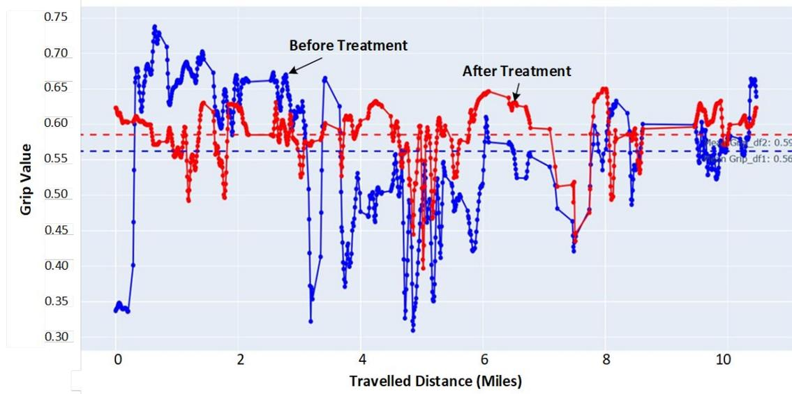
**Figure 3-3: Grip values before and after treatment for the auto-grip mode**
