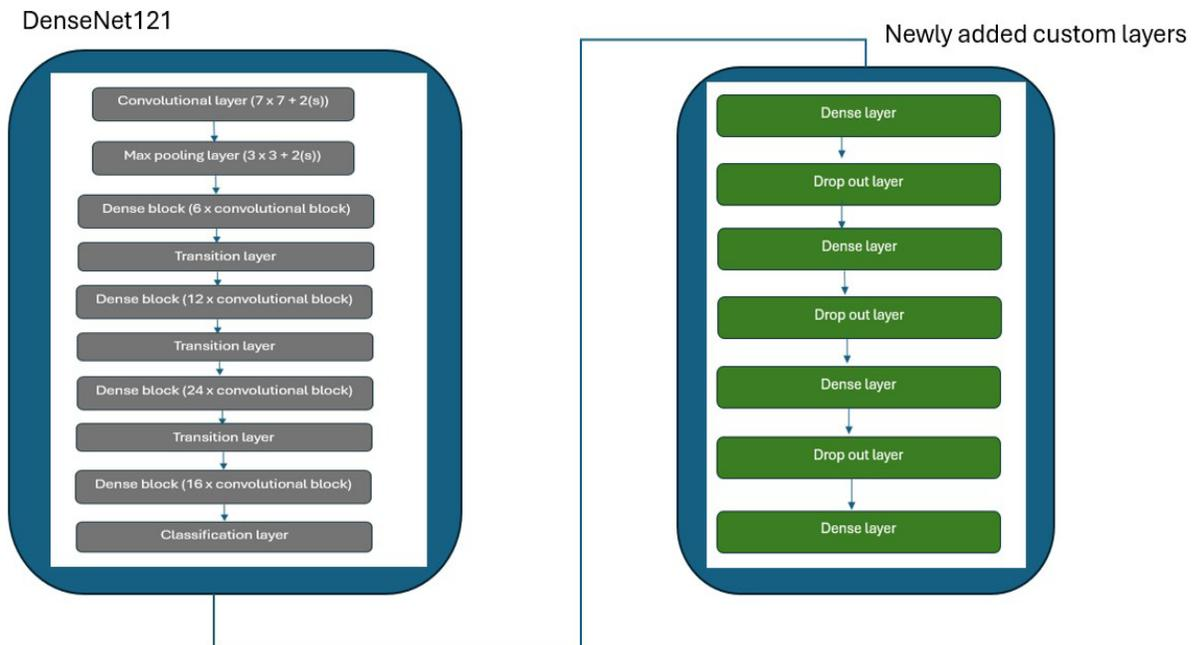
**Figure 2-14: Architecture of the RSC model using DenseNet121**
