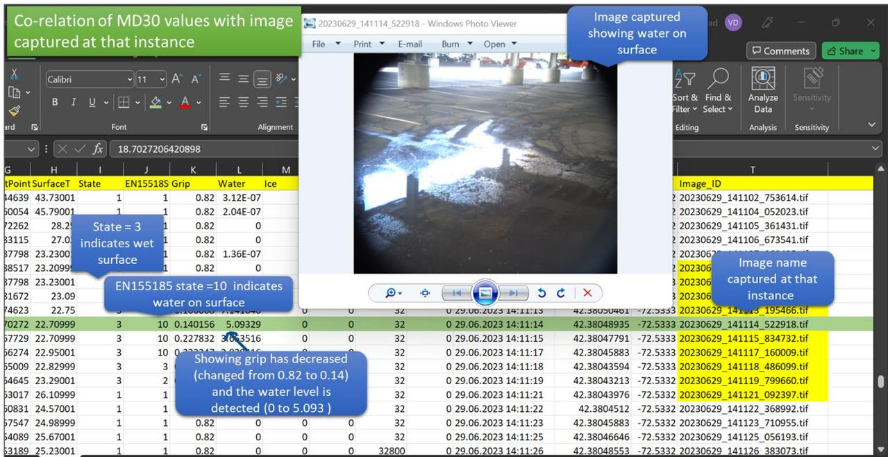
Figure 2-11: Sample data from the developed software
