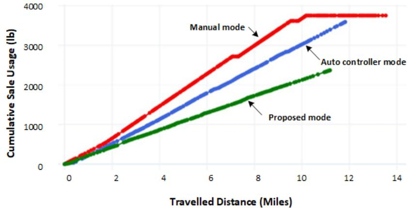
**Figure 3-6: Cumulative salt on roads during auto-grip, manual, and proposed modes**
