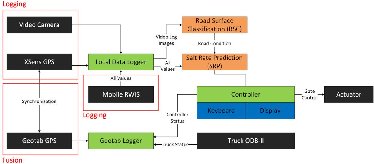
**Figure 2-10: Software development for the new system**
