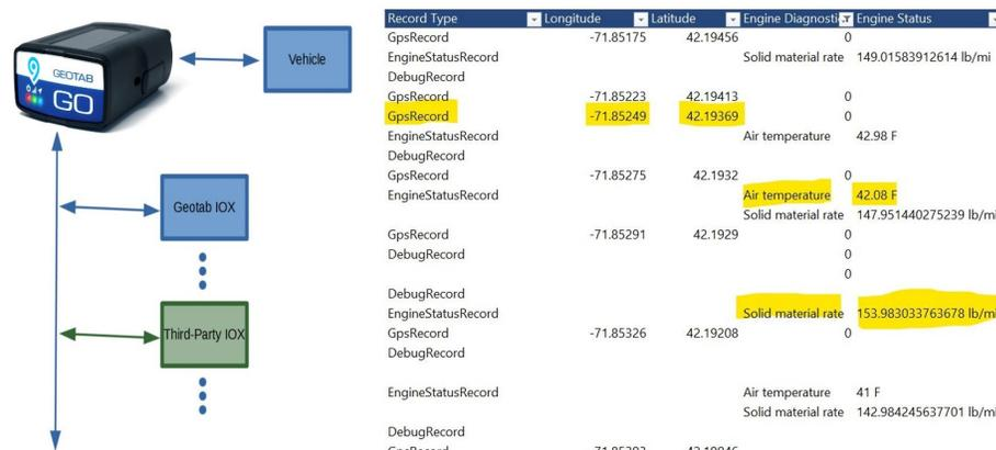
**Figure 2-6: Geotab logger and the recorded sample data**
