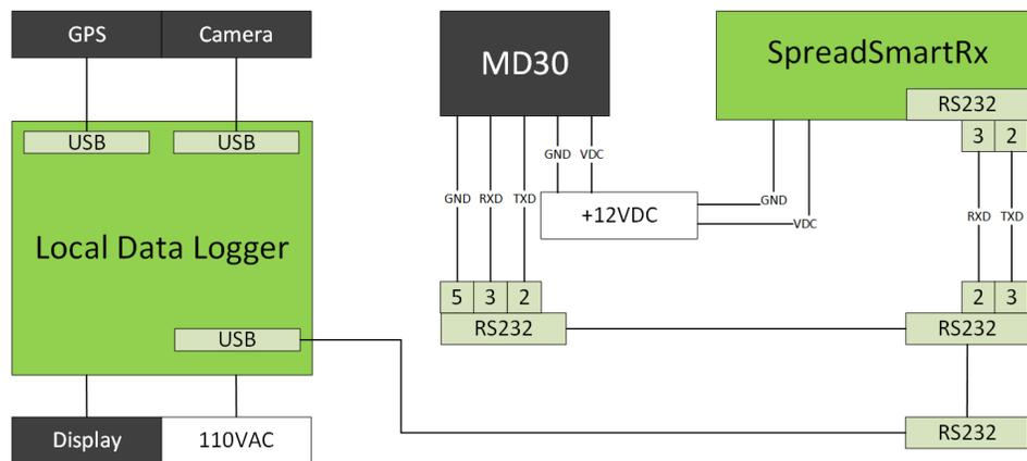
**Figure 2-8: Data I/O and power supply schematics**
