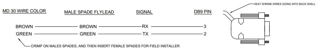
**Figure 6-11: MD30 to SpreadSmartRx connection**
