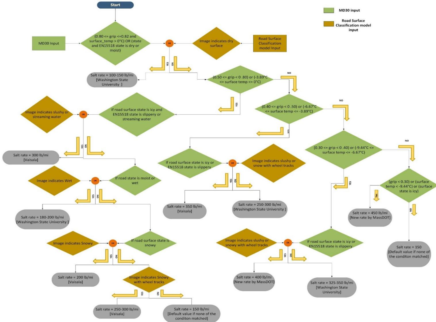
Figure 2-17: SRP model for surface treatment
