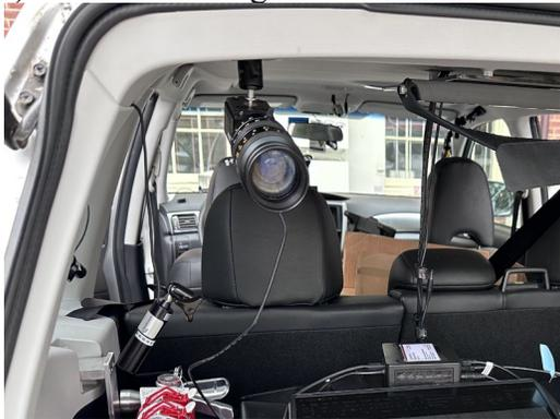
(c) Camera mounting on a SUV
