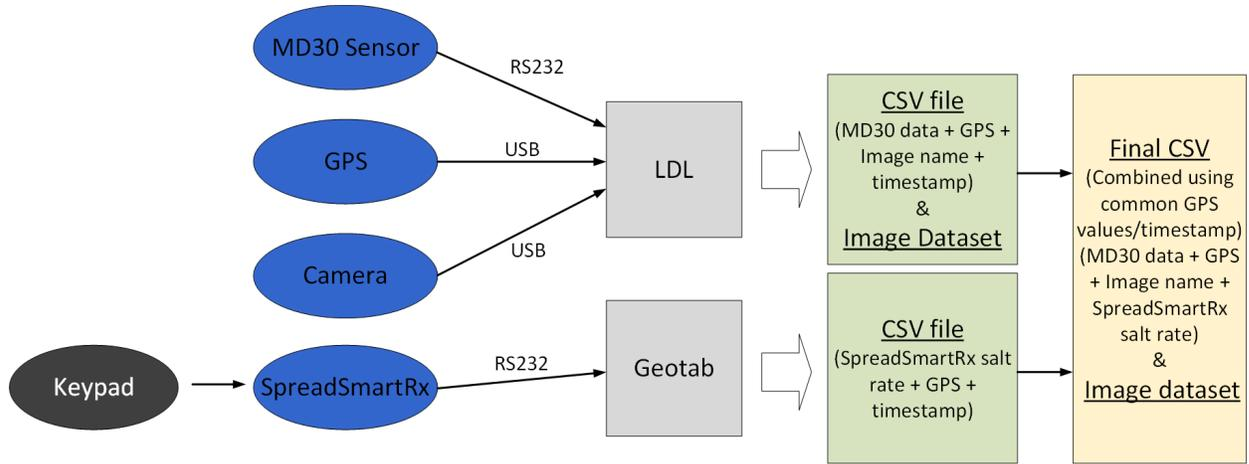
**Figure 2-12: Data fusion schematic from the LDL and Geotab**
