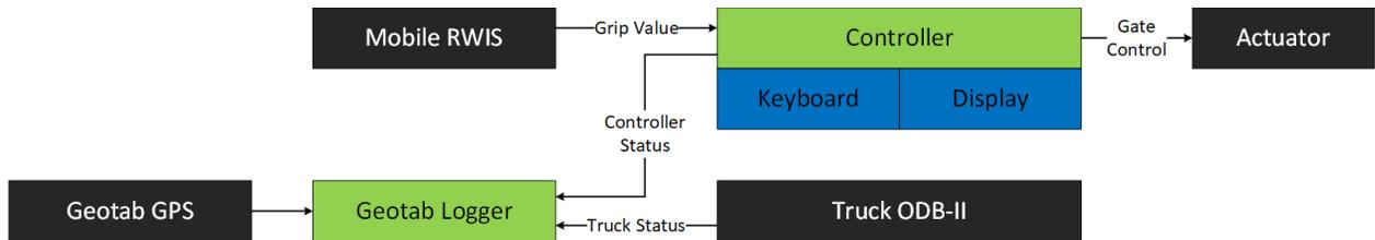
**Figure 2-3: Sensor and data logging systems on the MassDOT truck**
