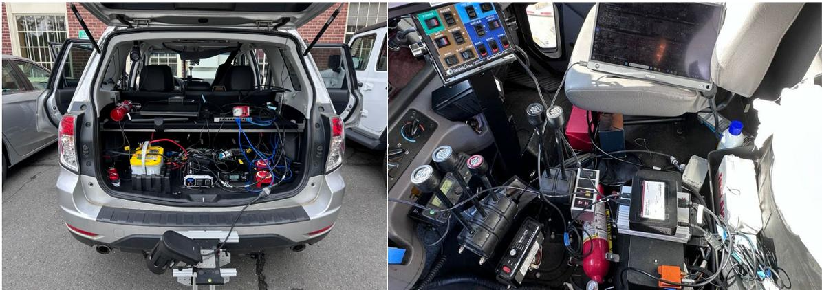
**Figure 2-9: Hardware on the UMass vehicle (left) and the MassDOT truck (right)**
