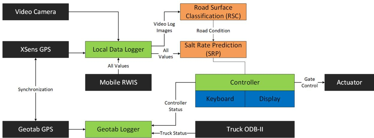
Figure 2-2: High-level block diagram of salt spreader system
