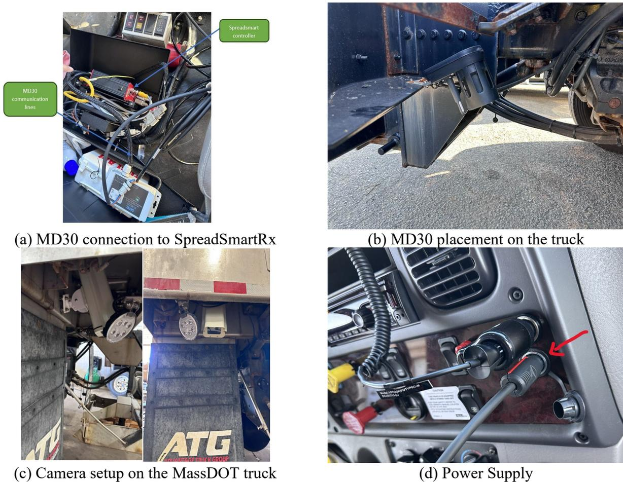
**Figure 6-7: Installed sensors on the MassDOT Truck**
