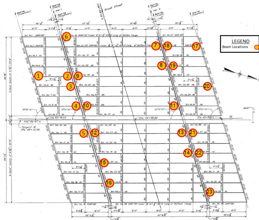
Figure 3.2. Example scanning plan for a highway bridge
