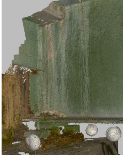
Figure 5.3. Registration SEKO (73) spheres on a corroded beam specimen.
