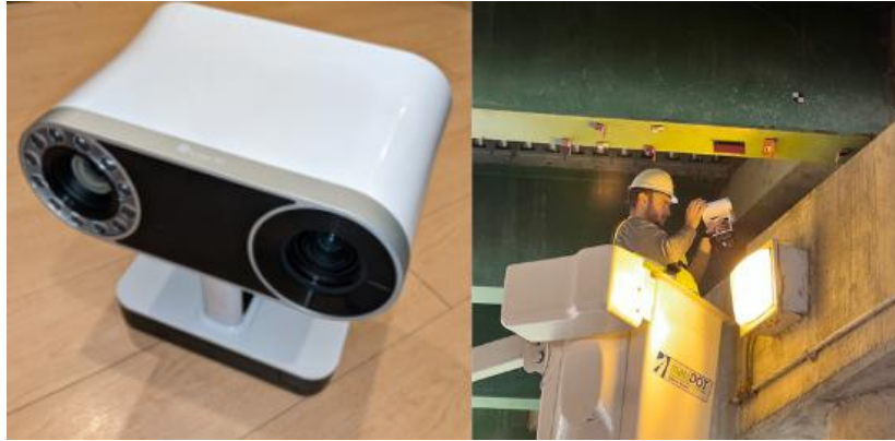
Left: the LEO scanner (70). Right: an inspector operating the LEO (70) and performing a beam end scan from a bucket truck on a highway bridge.
