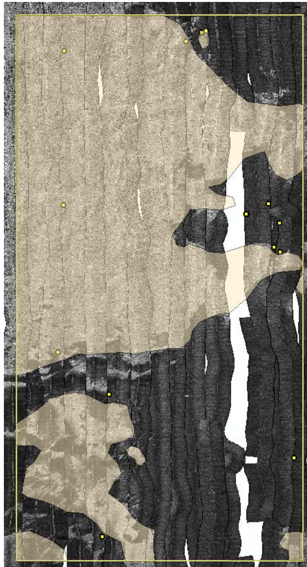
Figure 9: Side scan sonar mosaic of the pilot survey area (within the yellow box). Lighter shaded regions indicate high backscatter (complex habitat); darker shaded regions indicate low backscatter (simple habitat). Yellow dots are identified derelict pots.
