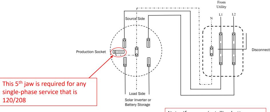
Note: If you are installing battery storage behind a production socket you will need a second disconnect on the load side of the production socket
