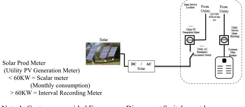
Note 1: Customer provided Emergency Disconnect Switch must be Located next to the Eversource Revenue meter and plainly marked.
