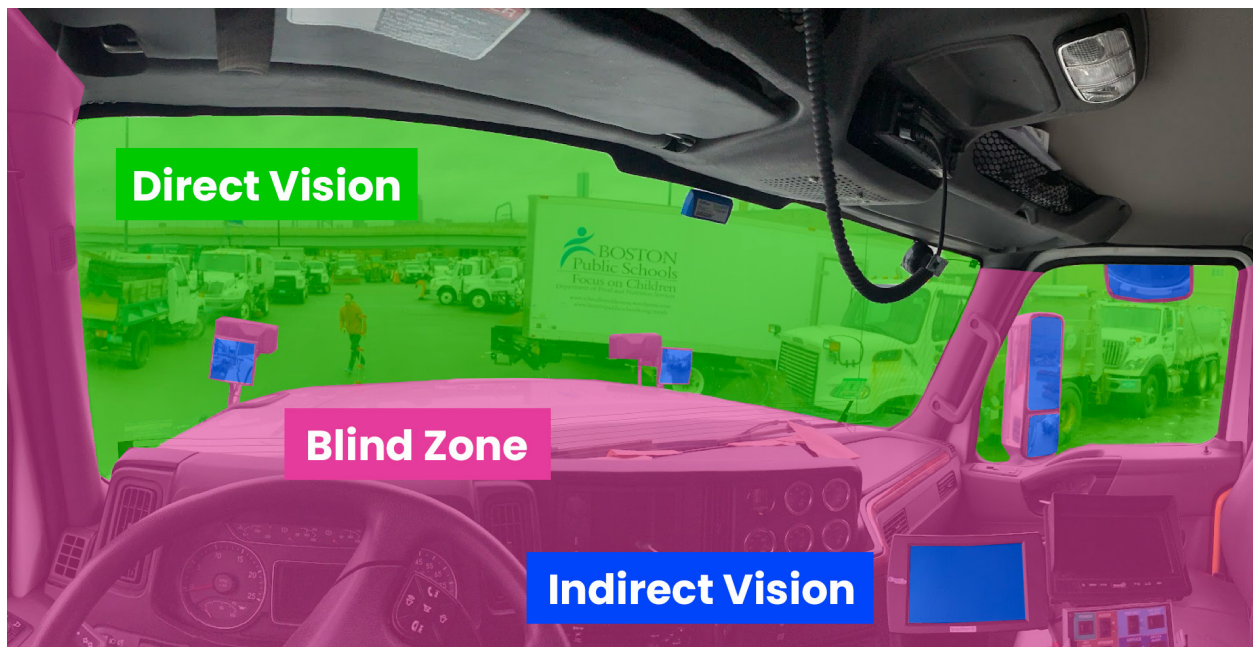
Figure 1: View from the driver's seat of an International HV 513. Direct vision of the environment is shaded green (unobstructed view through the windows), indirect vision areas are shaded blue (mirrors and camera display unit), and the blind zone areas are shaded in pink (hood, A and B pillars, and door).
