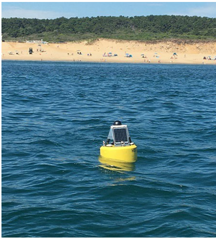
Figure 33. A real-time acoustic receiver deployed off Newcomb Hollow Beach, Wellfleet.
