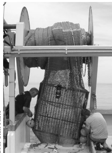
Fishermen Frank and Andrew Mirarchi (F/V Barbara L. Peters) adjust the floatation for the dogfish excluder grate. An underwater camera was attached to observe fish reactions.
