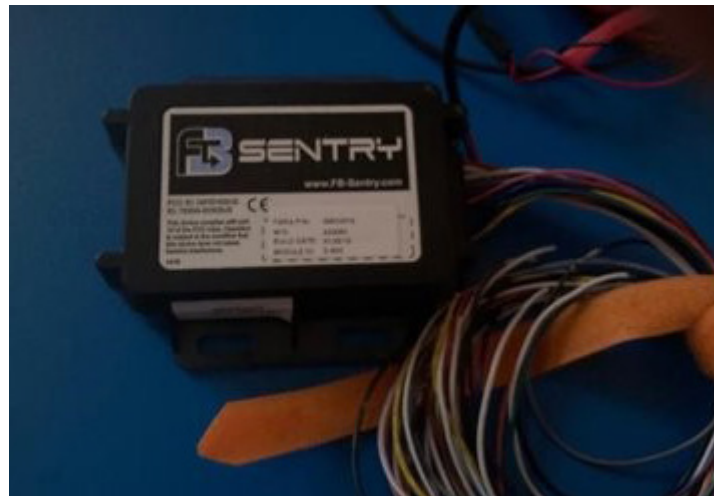
An example of the type of vessel tracker to be required in the lobster fishery.
