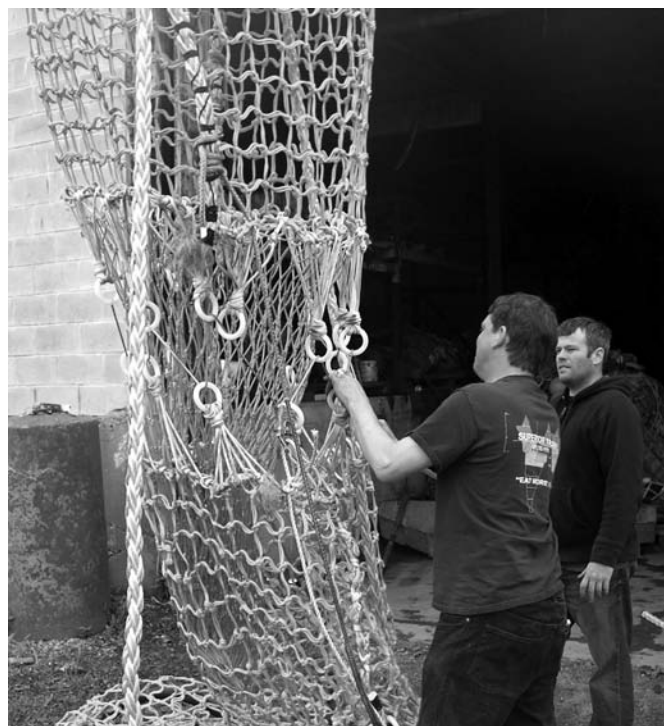
Jon Knight (left, Superior Trawl) and Dan Murphy (F/V Bantry Bay) inspecting the self-closing cod-end suspended from a crane truck.
