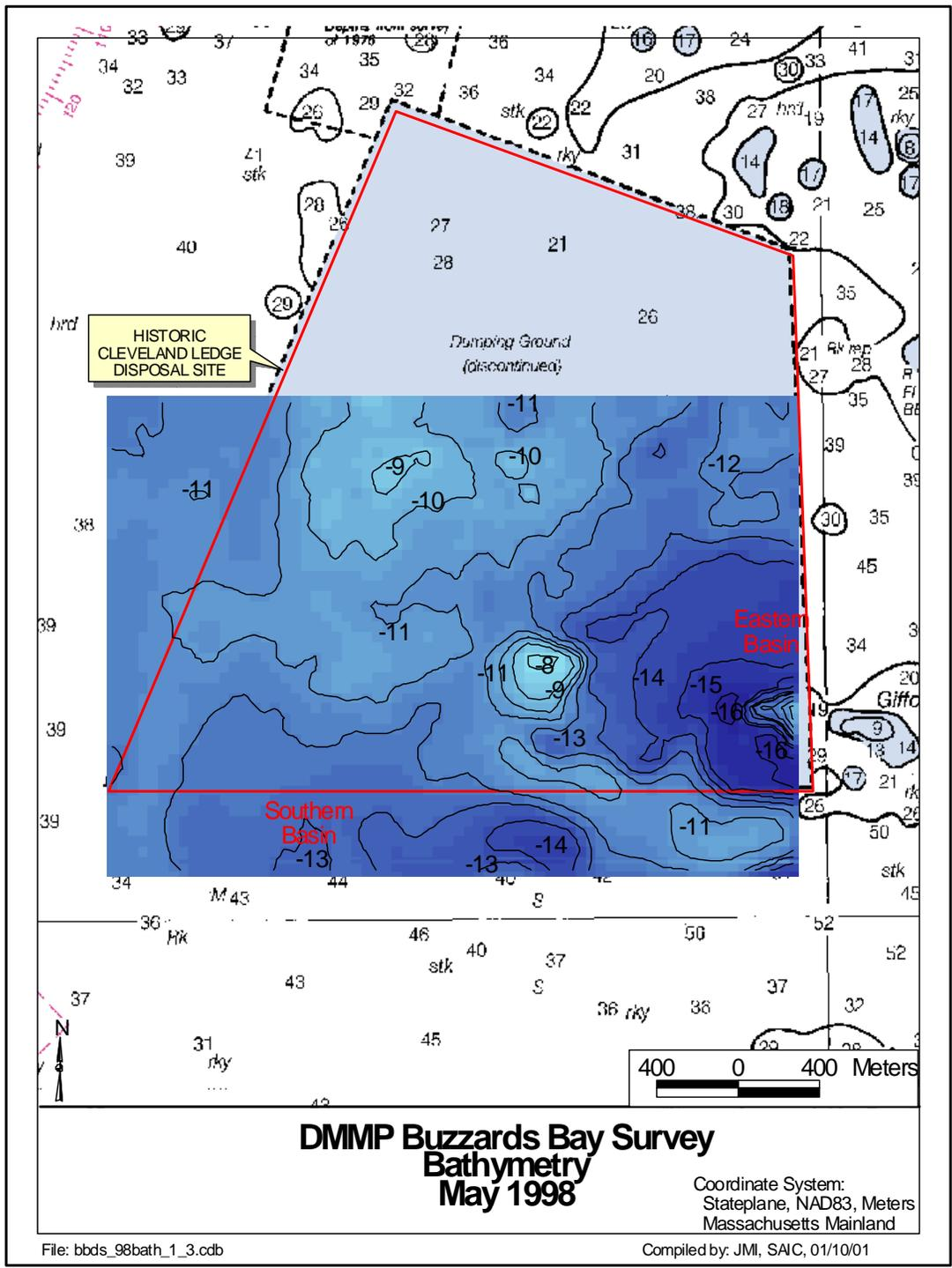
**Figure 1-3.** Results of the high-resolution bathymetric survey conducted across the southern half of the Cleveland Ledge Disposal Site in May 1998, superimposed on NOAA Nautical Chart 13229. Depths from the bathymetric survey are in meters; nautical chart depth soundings are in feet.
