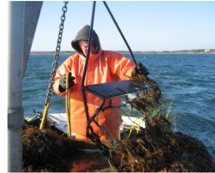
Dredge with pressure plate “pan dredge” in use on Vineyard in 2006 (MacKenzie 2008)
