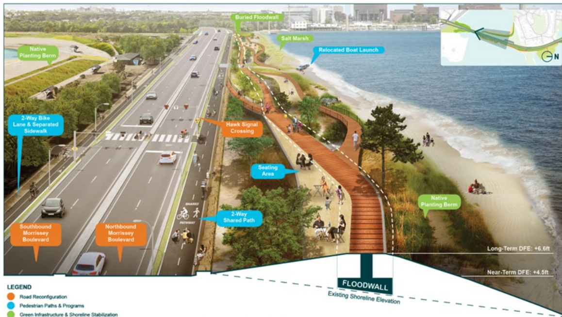
Figure 4-17: Buried Floodwall Option in the Central Section
