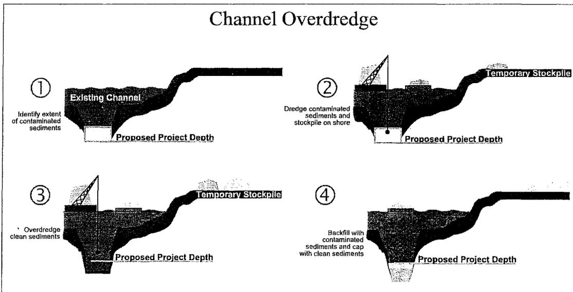
Figure 4-2: Schematic of Channel Overdredge (OD) method
