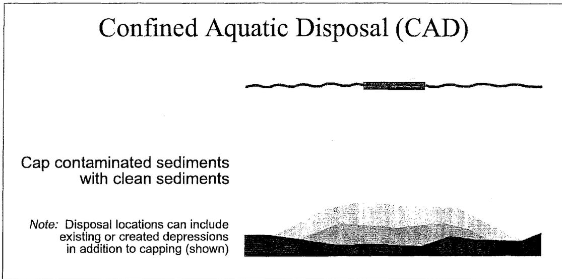
Figure 4-1: Schematic of Confined Aquatic Disposal (CAD) Method
