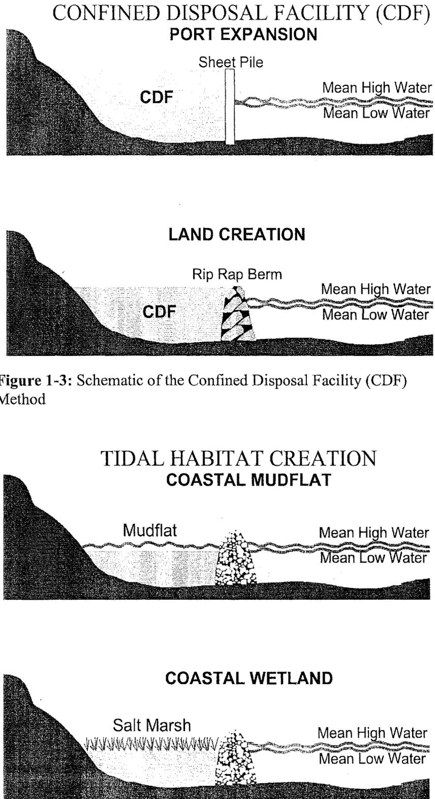
Figure 1-3: Schematic of the Confined Disposal Facility (CDF) Method
