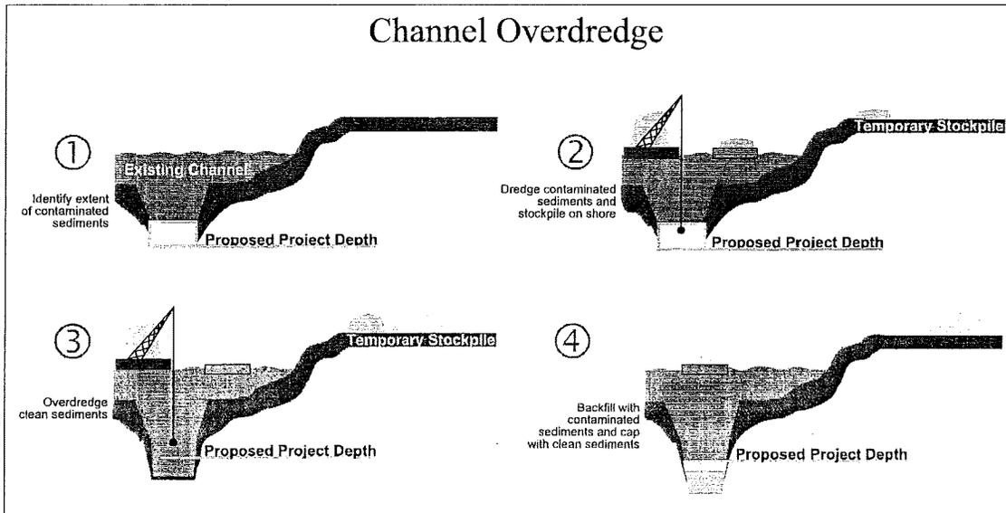
Figure 1-2: Schematic of Channel Overdredge (OD) method
