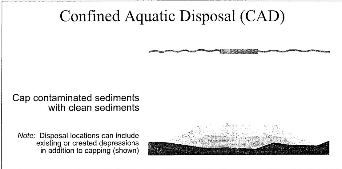
Figure 1-1: Schematic of Confined Aquatic Disposal (CAD) Method
