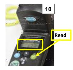
Repeat steps 5-6. Press Read (√) button. Result will display. If chlorine residual is not typical, retest with a fresh sample or contact Supervisor.
