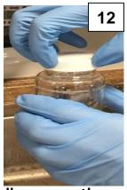
Carefully remove the cap. Keep threads facing down. Never put the cap down. Do not touch the threaded areas. Discard & fill a replacement bottle if contamination is suspected.
