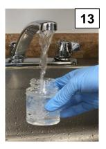
Fill coliform bottle to the shoulder, above the 100mL line. Do not overfill the bottle as this will remove the preservative.
