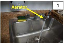
Inspect area at the designated sample site & tap. Remove the aerator and any attachments (e.g., hoses, tubing).
