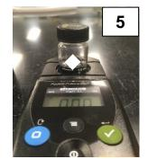
Wipe down sample cell. Place in colorimeter with diamond facing toward you.
