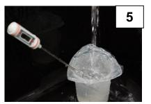
Place a thermometer into a sampling cup under the water flow. Continue flushing until temperature is stable.
