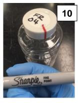
Label the cap of the coliform bottle with waterproof marker to match the "Type & Code" on the COC form. This describes the community and location sampled.
