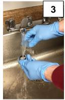
Use tap water to rinse the glass sample cell and cap 3 times.
