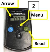
If needed, toggle to LR channel by pressing Menu then Read (✓) until arrow is under LR.
