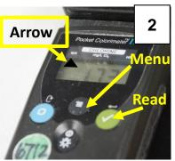
If needed, toggle to MR Use tap water to channel by pressing Menu then Read (√) until arrow is under MR.
