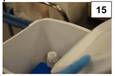
Immediately place sample into a dedicated drinking water sampling cooler with an ice pack. Do not use wet ice! Transfer sample(s) to laboratory. The hold time is 30 hours for a chlorinated sample.
