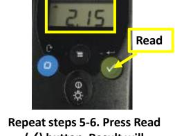
(√) button. Result will display. If chlorine residual is not typical, retest with a fresh sample or contact Supervisor. If result is blinking 2.20, retest on HR.
