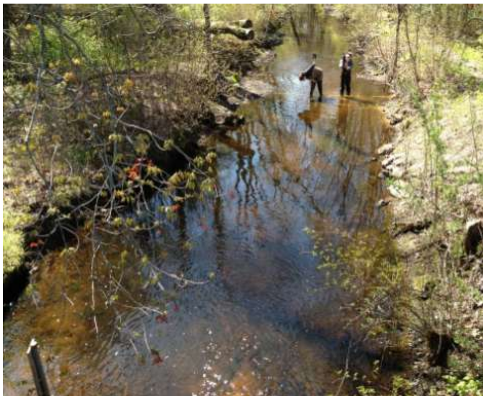
RIFLS staff measure flow downstream of the newly-installed staff gage (see lower left corner) on River Meadow Brook in Carlisle.
