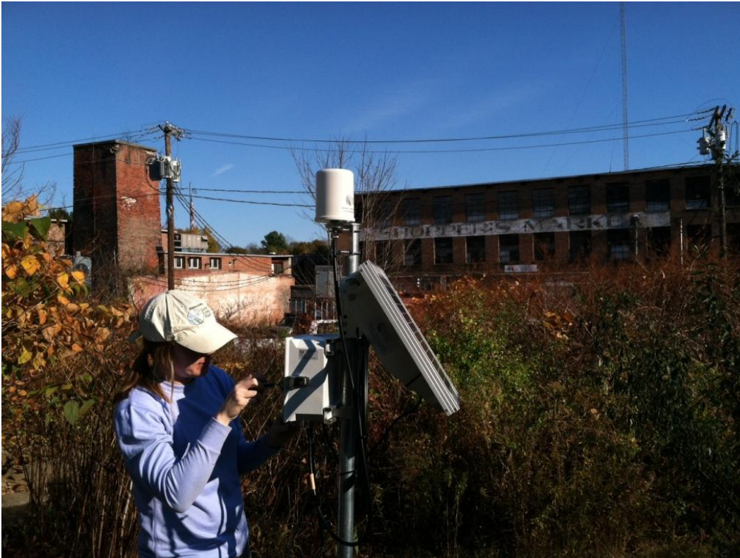
RIFLS staff install a solar powered telemetry station on Pecks Brook that transmits water level data in real time.
