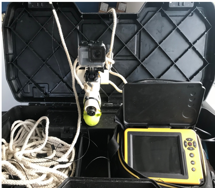
Figure 6. GoPro & Aqua-Vu camera system mounted on weight. The Aqua-Vu camera includes the screen seen in the image. The AquaVu has a live feed to the surface so we can verify that the camera made it to the bottom and we can assign a preliminary seafloor interpretation.
