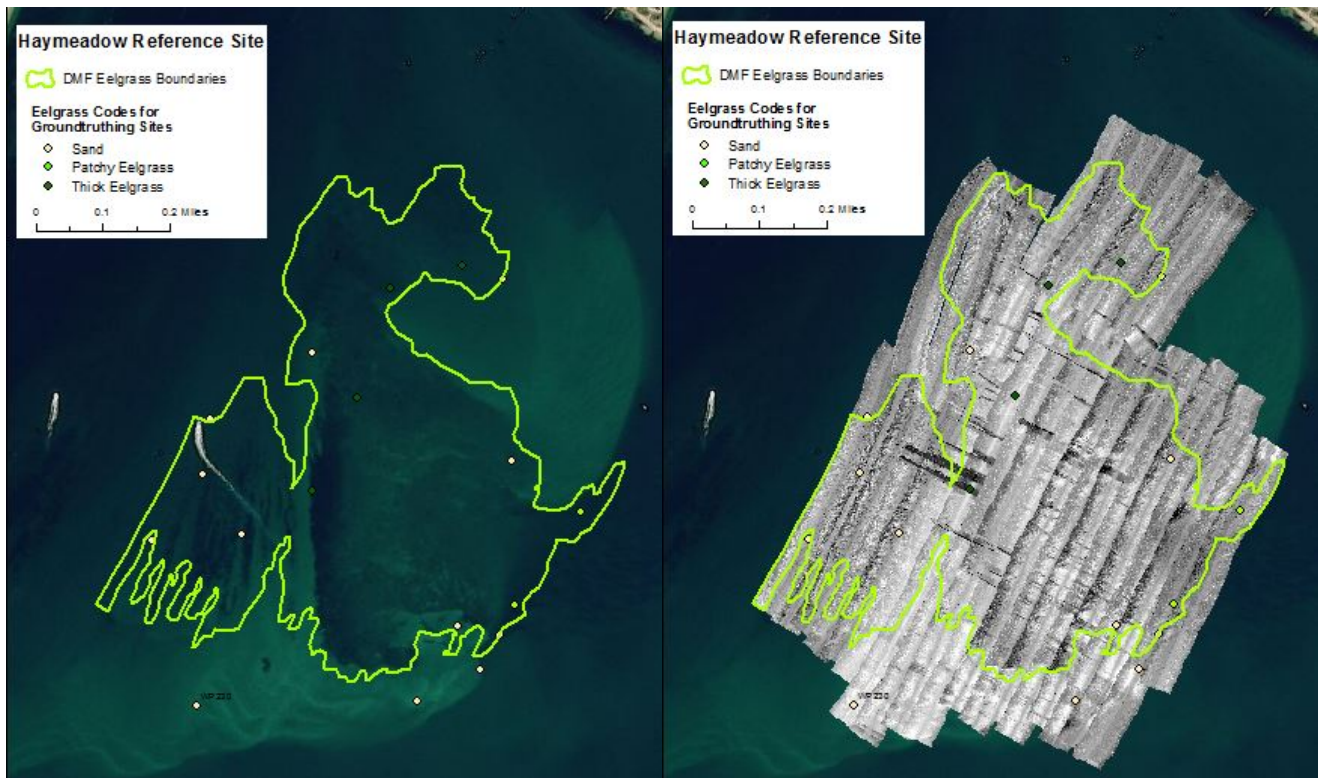
Figure 12. Aerial imagery from Sept 2018 (left) and the sonar mosaic with groundtruthing points from Aug 2019 (right). The eelgrass delineation done with the 2019 side scan sonar data is overlaid on both images as a green line.
