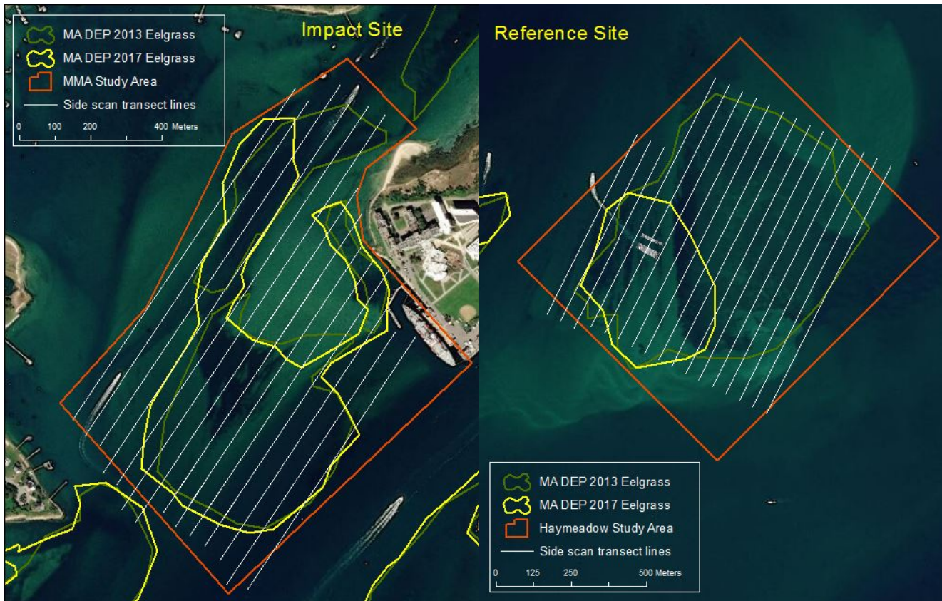
Figure 5. Planned transect lines at the MMA impact and Haymeadow reference eelgrass meadow sites on Sept 2019 aerial imagery basemap.
