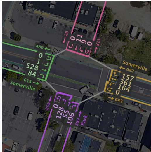
Figure 4.16: Bicycle turning movement counts at Somerville Avenue and Park Street, Somerville (11/19/2020 at 4:00 p.m. to 11/20/2020 at 4:45 p.m.)
