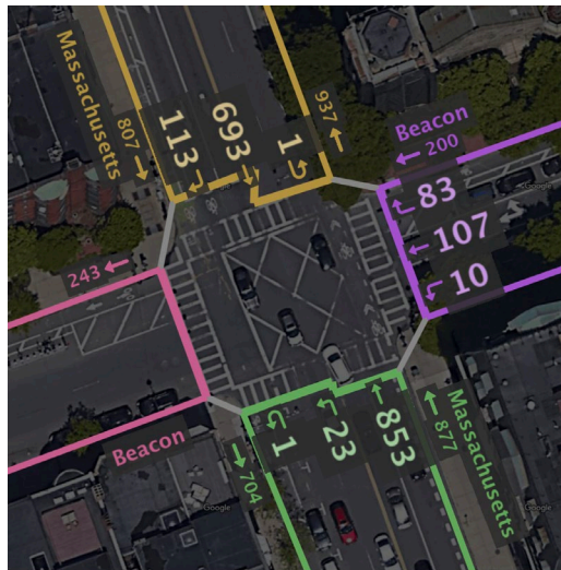
Figure 4.11: Bicycle turning movement counts at Beacon St. and Massachusetts Ave. (11/2/2020 at 12:30 p.m. to 11/3/2020 at 1:15 p.m.)
