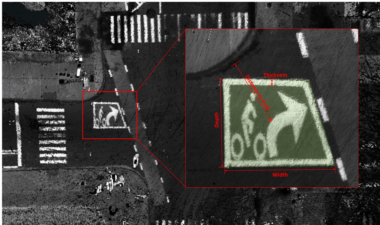
Figure 2.4: Illustration of TSTQB dimensions using LiDAR point cloud
