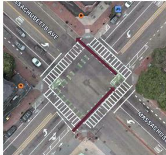
(b) Two-stage turn maneuver using the TSTQB (Image source: Google)
