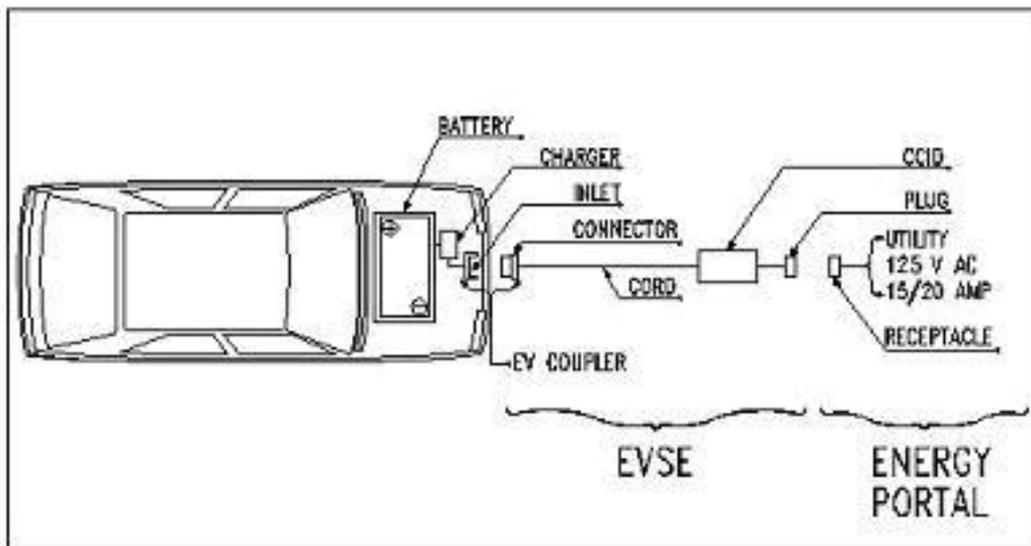
EV suppliers provide a Level 1 Cord Set (120 VAC, 15 or 20 amps) with the vehicle. The Cord Set uses a standard 3-prong plug (NEMA 5-15P/20P) with a charge current interrupting device (CCID) located in the power supply cable within 12 inches of the
