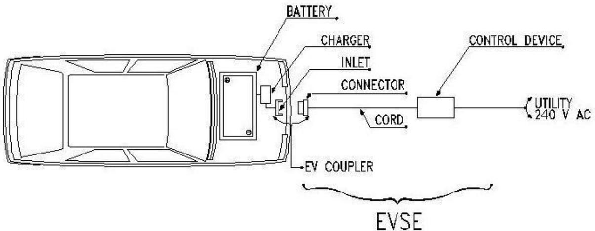
The higher voltage of Level 2 allows a much faster battery charge. Because of the higher voltage, Level 2 has a higher level of safety requirements than Level 1 under the NEC, including the requirement that the connector and cord be hardwired to the control device and premises wiring.
