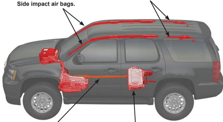
**DO NOT CUT HERE.** Under vehicle area near passenger side frame rail contains high voltage 300 volt electrical cables.
