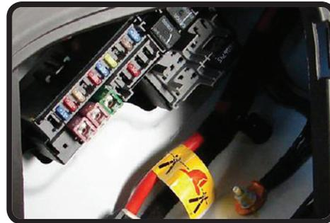
Cut through the red positive low voltage cable on each side of the tag to remove a section of the cable to ensure the cables cannot inadvertently reconnect.
