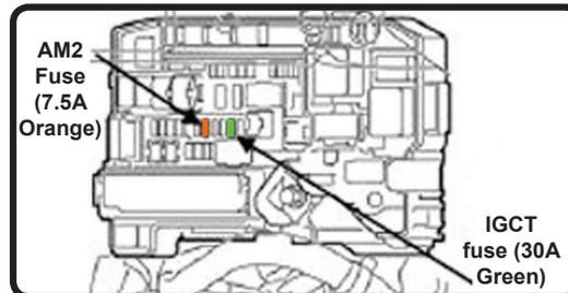
IGCT and AM2 Fuse Location In Engine Compartment Fuse Box
