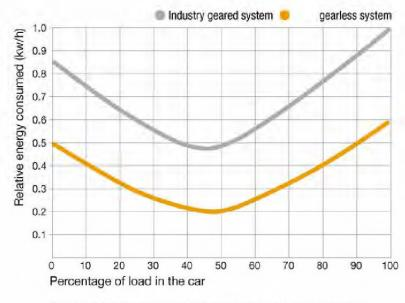
Based on 3500 lb. system at 350 feet per minute at 180 starts per hour.
