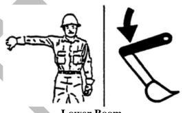
**Lower Boom**With either arm extended horizontally, fingers closed, point thumb downward.
