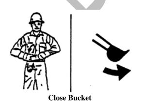
Hold one hand closed and stationary. Rotate other hand in small vertical circle with forefinger pointing horizontally at closed hand.
