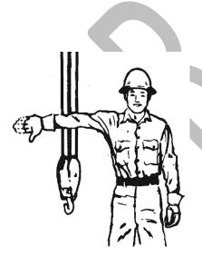
Lower the Boom and Raise the Load With arm extended, thumb pointing down, flex fingers in and out as long as load movement is desired.
