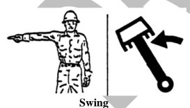
With either arm extended horizontally, point with forefinger to direction of swing rotation.
