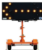
Right lane closure - merge left
