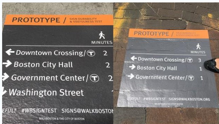
WalkBoston has also been testing wayfinding pavement decals in downtown Boston - designed for areas with no available sign poles - in order to determine their durability. Source: WalkBoston
