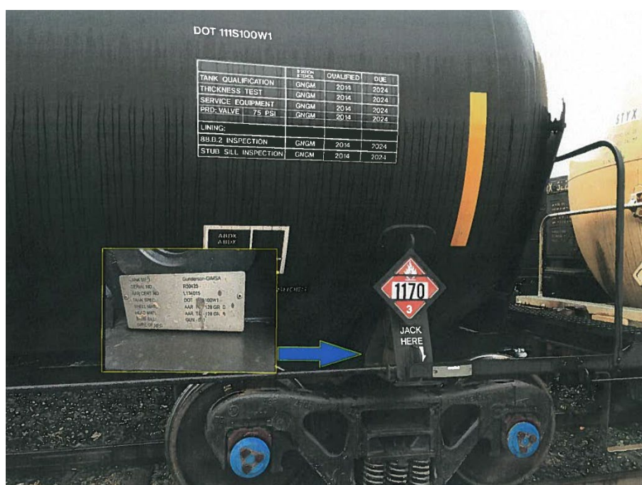
Figure 3 – Location of a tank car identification plate. This can be found on the bolster web at the left side of the B End (courtesy Providence and Worcester Railroad).
