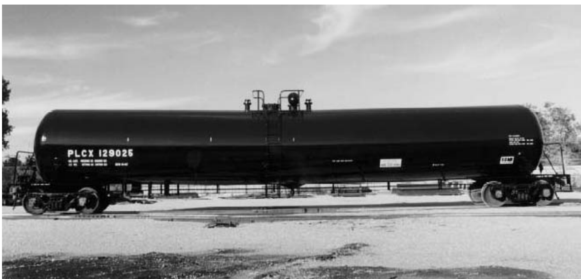
Figure 1 – Rail tank car typically used to carry ethanol and similar products. The tank car's initials and car number are shown at the left side (PLCX 129026). This car's capacity is 29,815 gallons and the exterior length is 67 feet, 11 inches.
