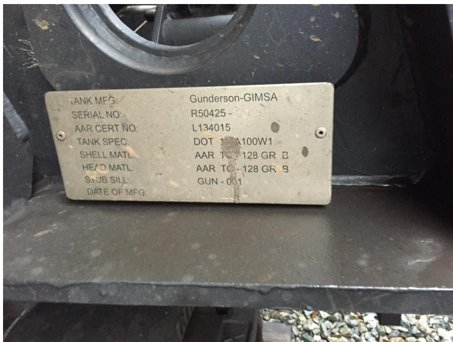
Figure 4 – Close-up of an identification plate. This shows the tank car manufacturer and the car’s serial number on the first two lines (courtesy Providence and Worcester Railroad).
