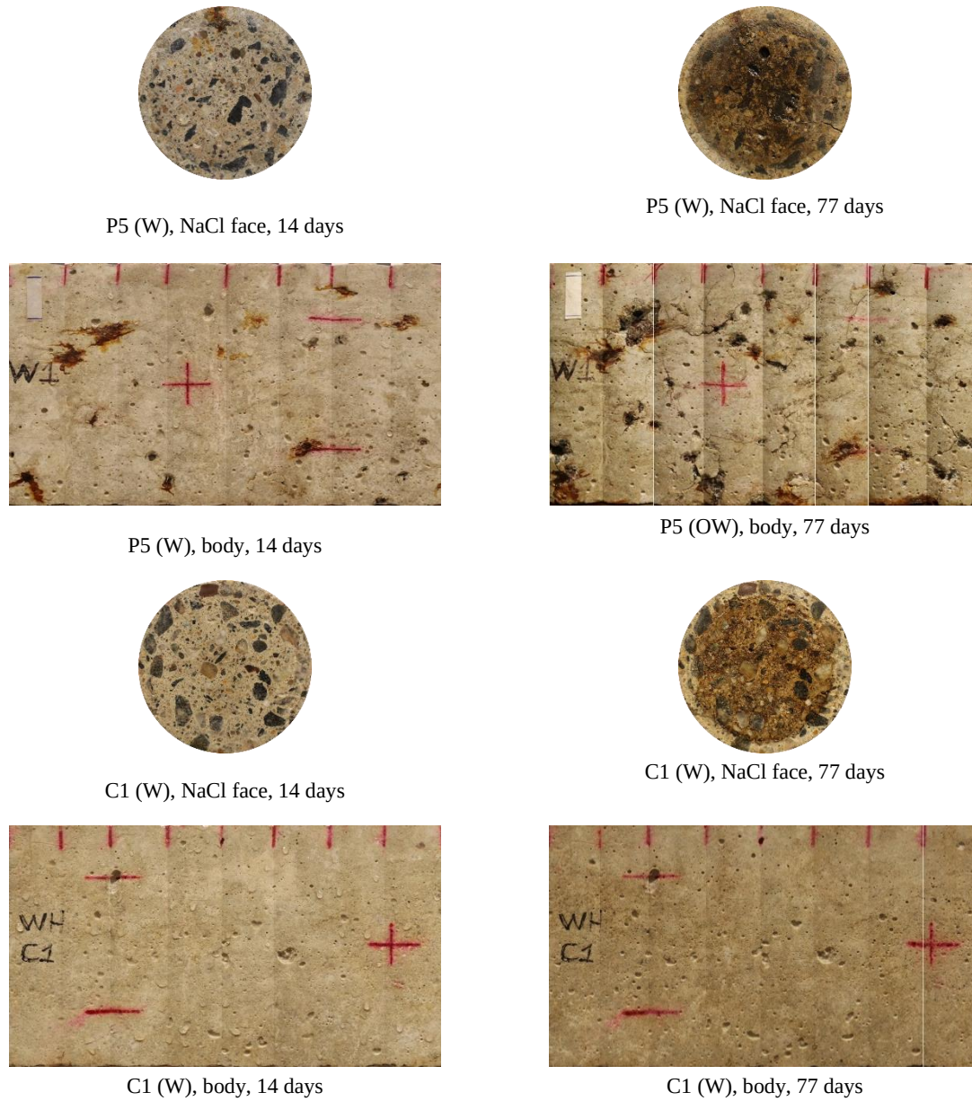
Figure 5 Crack evolution of G2 specimens for White cement at early stages and end of exposure.
