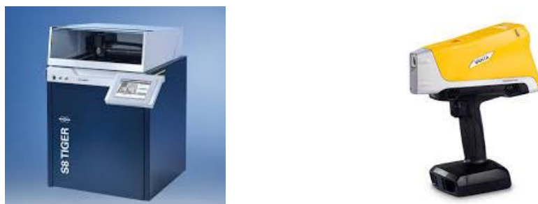
Figure 3: WDXRF (left) and EDXRF (right) instruments available in the UConn laboratories
