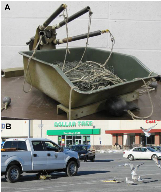
Figure 2. (A) The Coda net launcher used to capture gulls in Massachusetts, USA, 2008–2012. (B) A typical capture set-up in an urban parking lot. The net launcher was placed under the side of the truck and a pile of bait was placed in front. The launcher was detonated from inside the truck cab.
