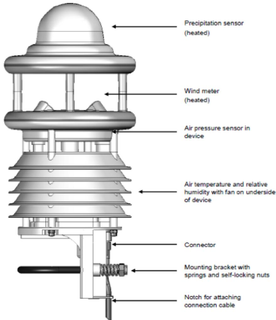
**Figure 3.8: Hardware structure of Lufft Compact Weatherstation WS600-UMB**
