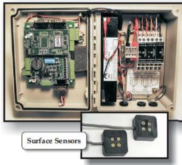
**Figure 2.9: High Sierra 5721 RWIS Road Sensor Station**
