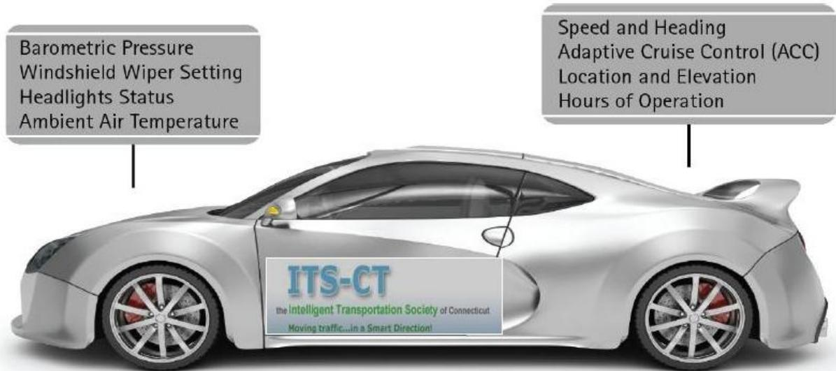
**Figure 2.6: Prototype RWIS-enabled vehicle under consideration in Connecticut**
