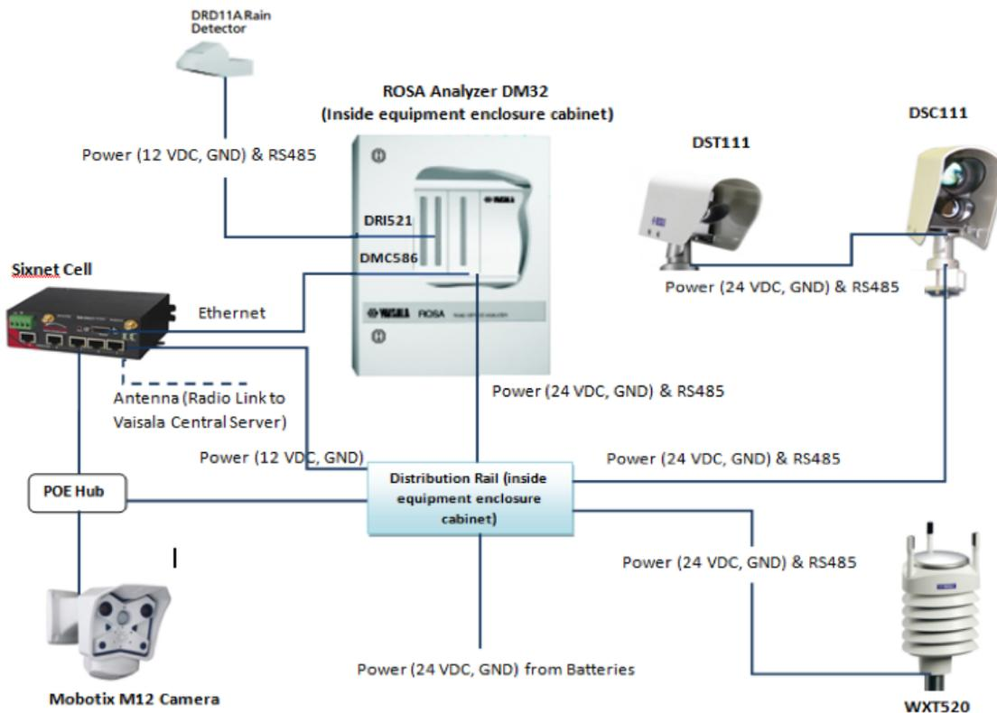
Figure 3.1: Connectivity diagram of Vaisala RWIS components
