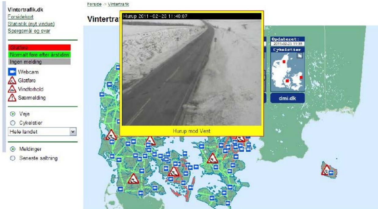
**Figure 2.1: Example of an RWIS-driven road weather application**
