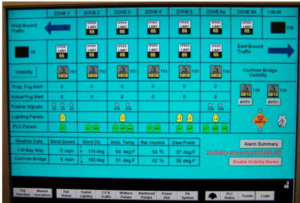
**Figure 2.5: Low-Visibility Warning System Interface**
