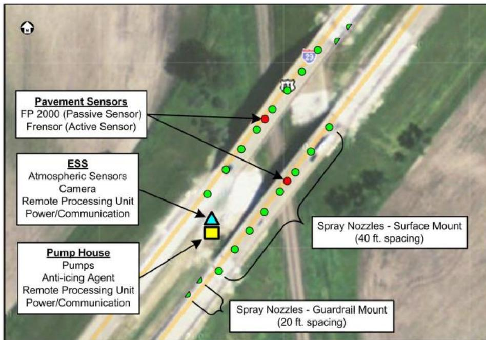
**Figure 2.7: I-29 Buxton Bridge FAST system components**
