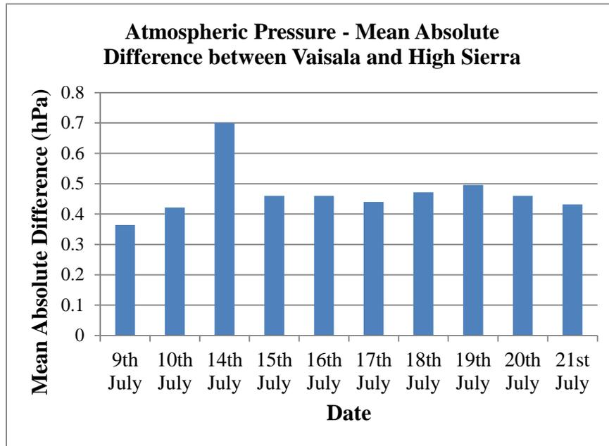
**Figure 3.15: Atmospheric pressure comparison**
