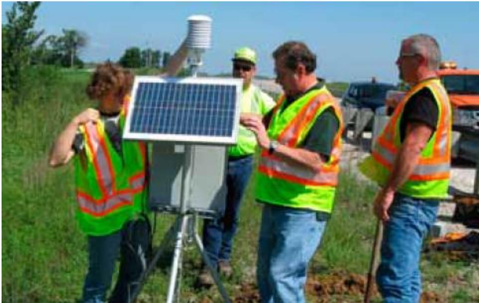
**Figure 2.10: Iowa portable RWIS**
