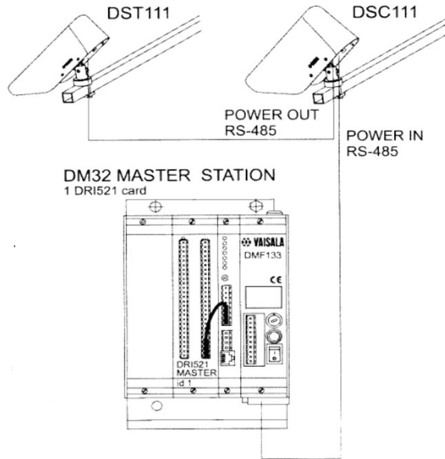
**Figure 3.2: DSC111 and DST111 connected to the ROSA analyzer**
