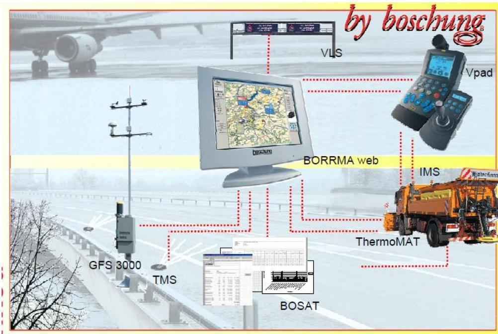
**Figure 2.2: Interconnection of RWIS and road maintenance components in Switzerland**
