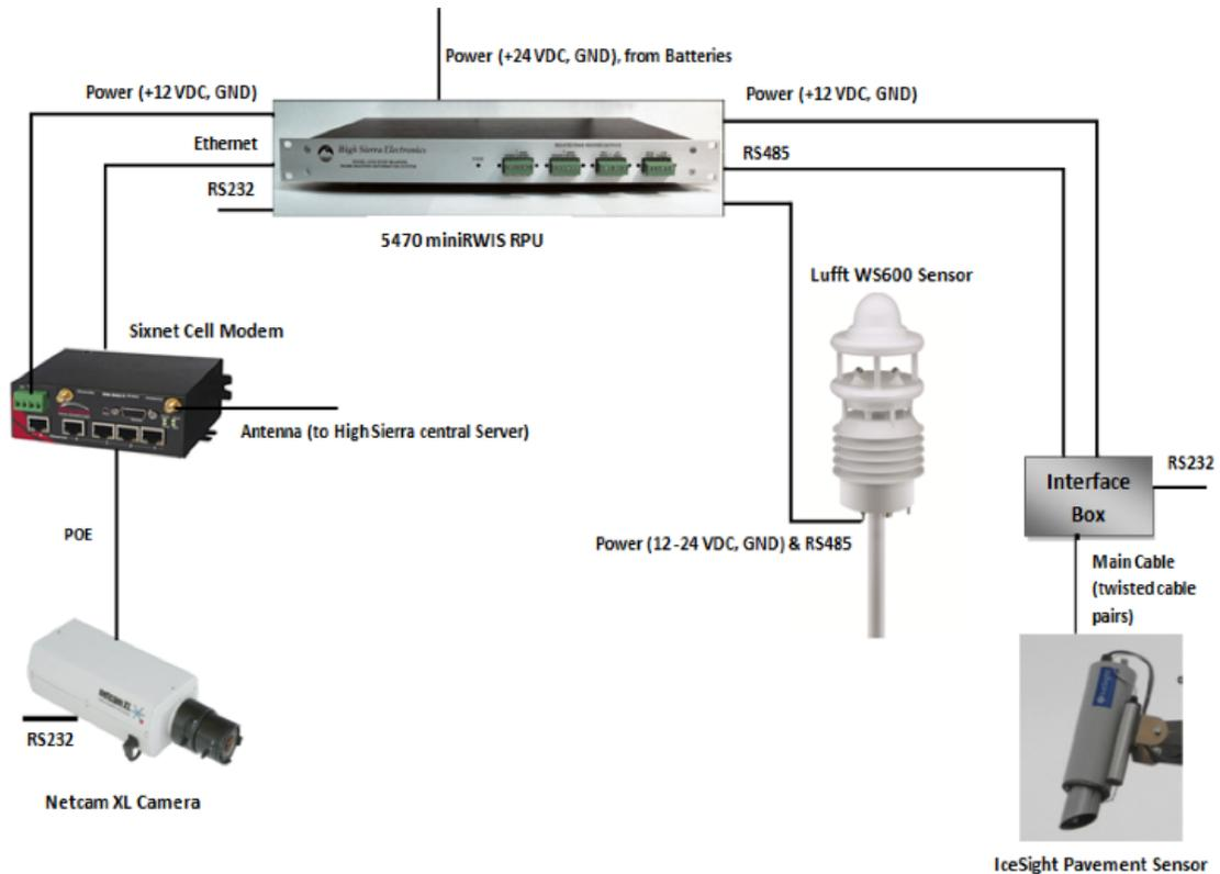
**Figure 3.6: Connectivity diagram of High Sierra RWIS**
