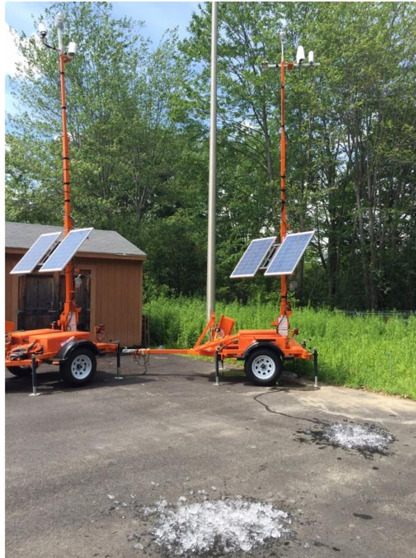
**Figure 3.25: Ice test performed at target detection spots for corresponding weather stations**
