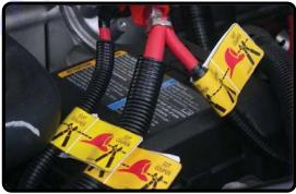
**Cut 3 Exposed Cables (Alternate Procedure)**
