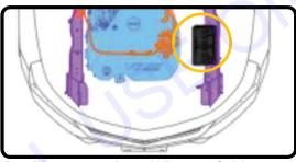
Disconnect the 12V Battery Cables
