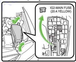
**Remove Fuse IG2 in Engine Compartment**
