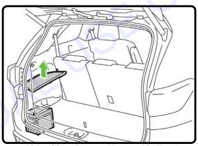
12V Auxiliary Battery Mounted in Trunk
