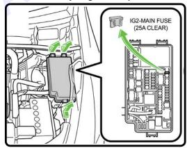
Remove Fuse IG2 in Engine Compartment
