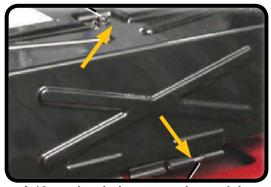
A 10 mm hex bolt secures the module. Hinges are attached to the battery cover.
