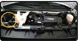
**Disconnect the 12V Battery Cables**
