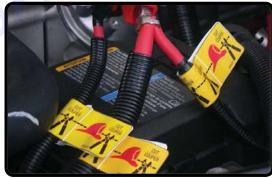
Cut 3 Exposed Cables (Alternate Procedure)
