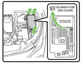
Remove Fuse IG2 in Engine Compartment
