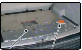
HV Battery Pack HV Service Disconnect Switch
