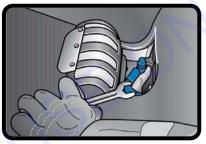
Disconnect the Ground at the Threaded Connection
