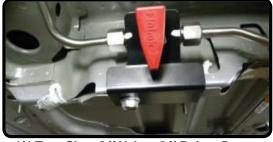
1/4 Turn Shut-Off Valve, Off Points Down
