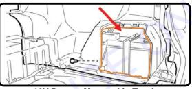
12V Battery Mounted in Trunk
