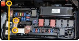
**Cut Cable and Main Fuse Screw Locations**
