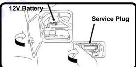
The low voltage battery is located in the trunk on the left side of the HV battery and is concealed by a trim cover.
