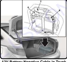
12V Battery Negative Cable in Trunk
