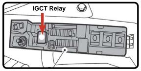
High Voltage Fuse and Fusible Link Box
