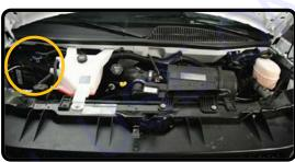
Disconnect the 12V Battery Cables
