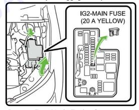
Remove Fuse IG2 in Engine Compartment
