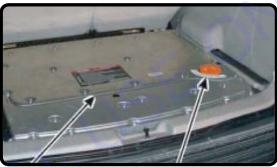
HV Battery Pack HV Service Disconnect Switch
