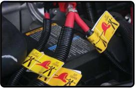
**Cut 3 Exposed Cables (Alternate Procedure)**
