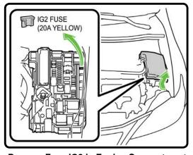
Remove Fuse IG2 in Engine Compartment
