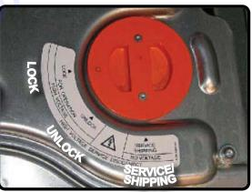
High-Voltage Service Disconnect Switch Shown in LOCK position
