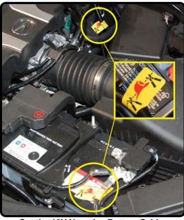
Cut the 12V Negative Battery Cable and DC to DC Converter Cable
