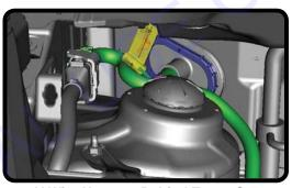
12V Wire Harness Behind Tower Strut, Engine Compartment, Passenger's Side
