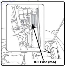
Remove Fuse IG2 in Engine Compartment
