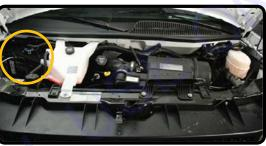
Disconnect the 12V Battery Cables
