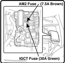
IGCT and AM2 Fuse Located in the Engine Compartment
