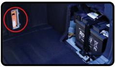
12V Battery and Service Plug in Trunk
