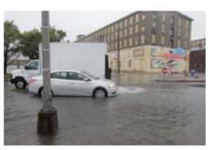
Chronic ponding/flooding in Stafford Square occurs due to the "bowl" shape of drainage basin and insufficient sewer and drain capacities.
