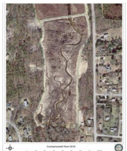
Image bottom: Coonamessett River in 2018 after Phase 1 restoration, note restored wetlands, the side channels, and stream connectivity due to removal of lower dam, replaced by a pedestrian boardwalk.
