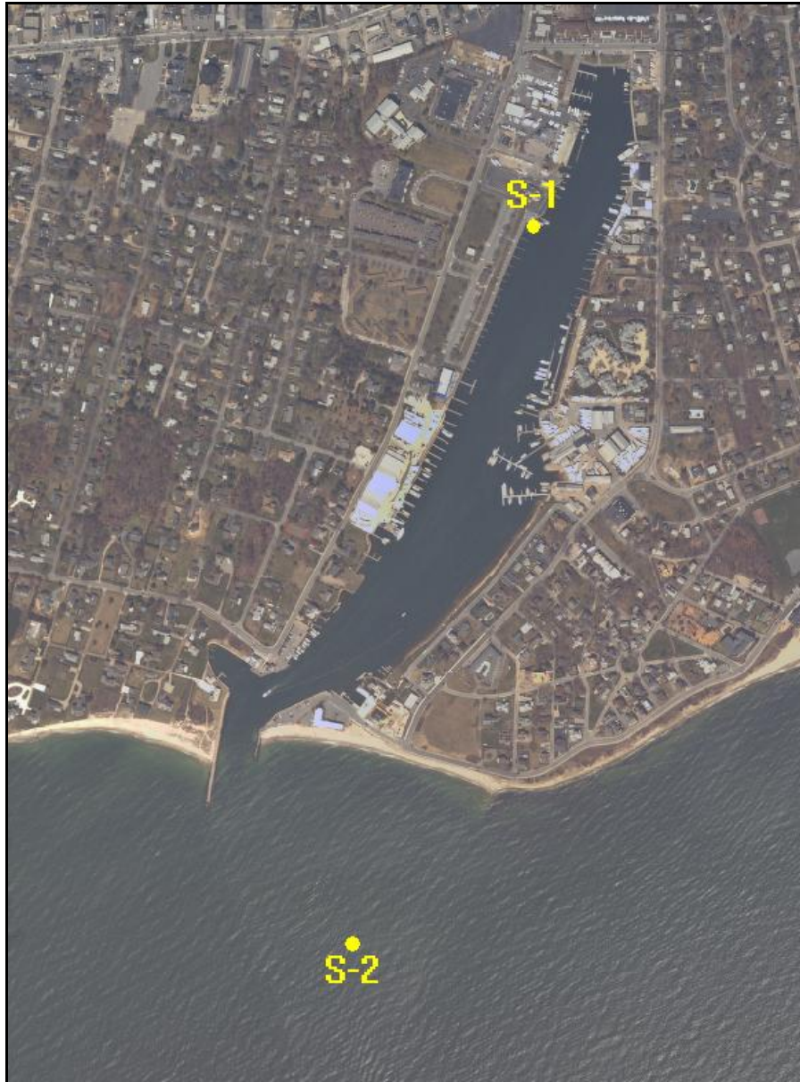
Figure V-2. Map of the study region identifying locations of the tide gauges used to measure water level variations throughout the system. The two (2) gauges were deployed for a 39-day period between April 22, and May 30, 2007. Each yellow dot represents the approximate locations of the tide gauges: (S-1) represents the Falmouth Inner Harbor gauge and (S-2) the Vineyard Sound gauge (Offshore).
