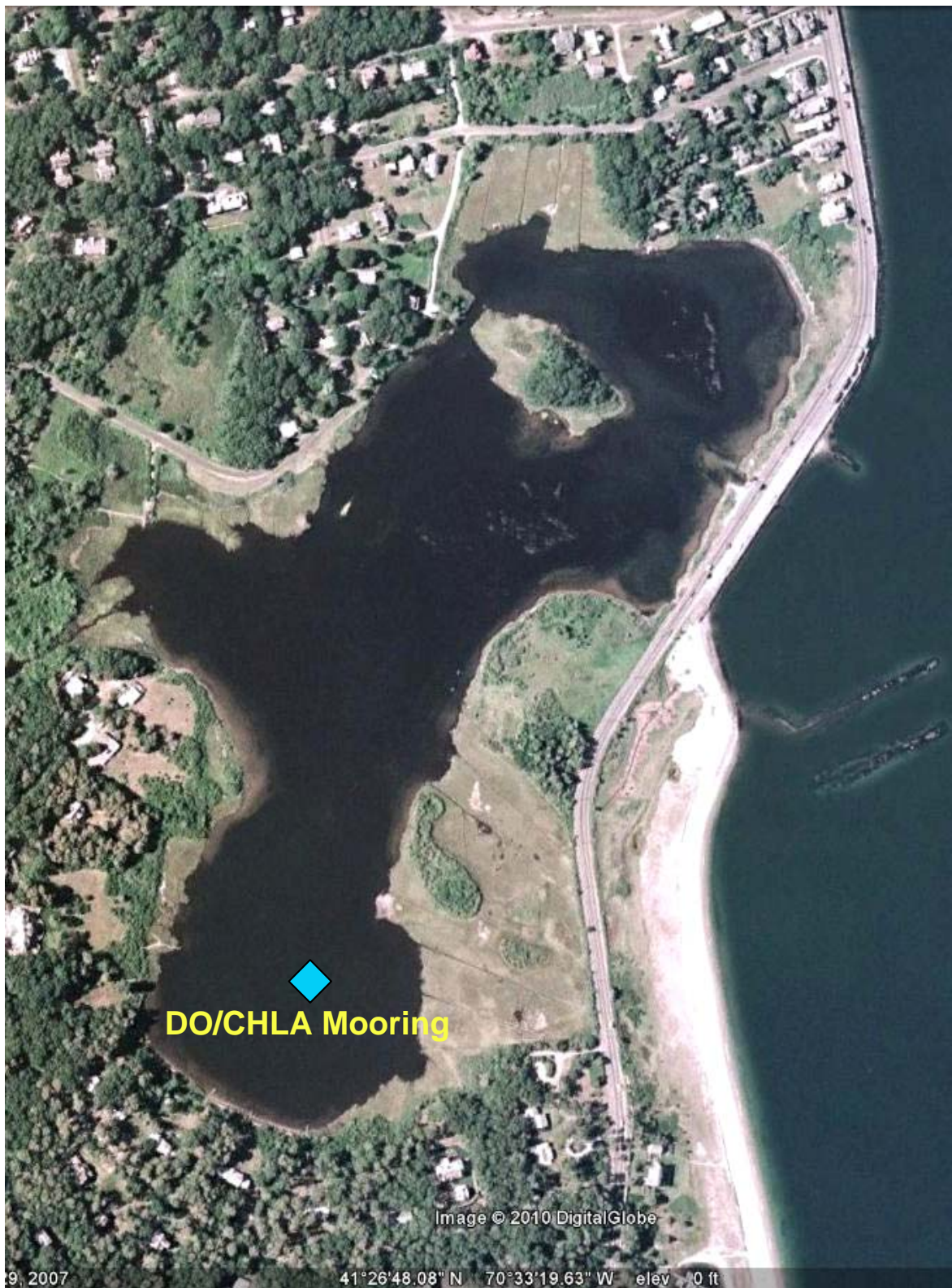
Figure VII-2. Aerial Photograph of the Farm Pond system in the Towns of Oak Bluffs showing the location of the continuously recording Dissolved Oxygen / Chlorophyll-a sensors deployed during the Summer of 2006.
