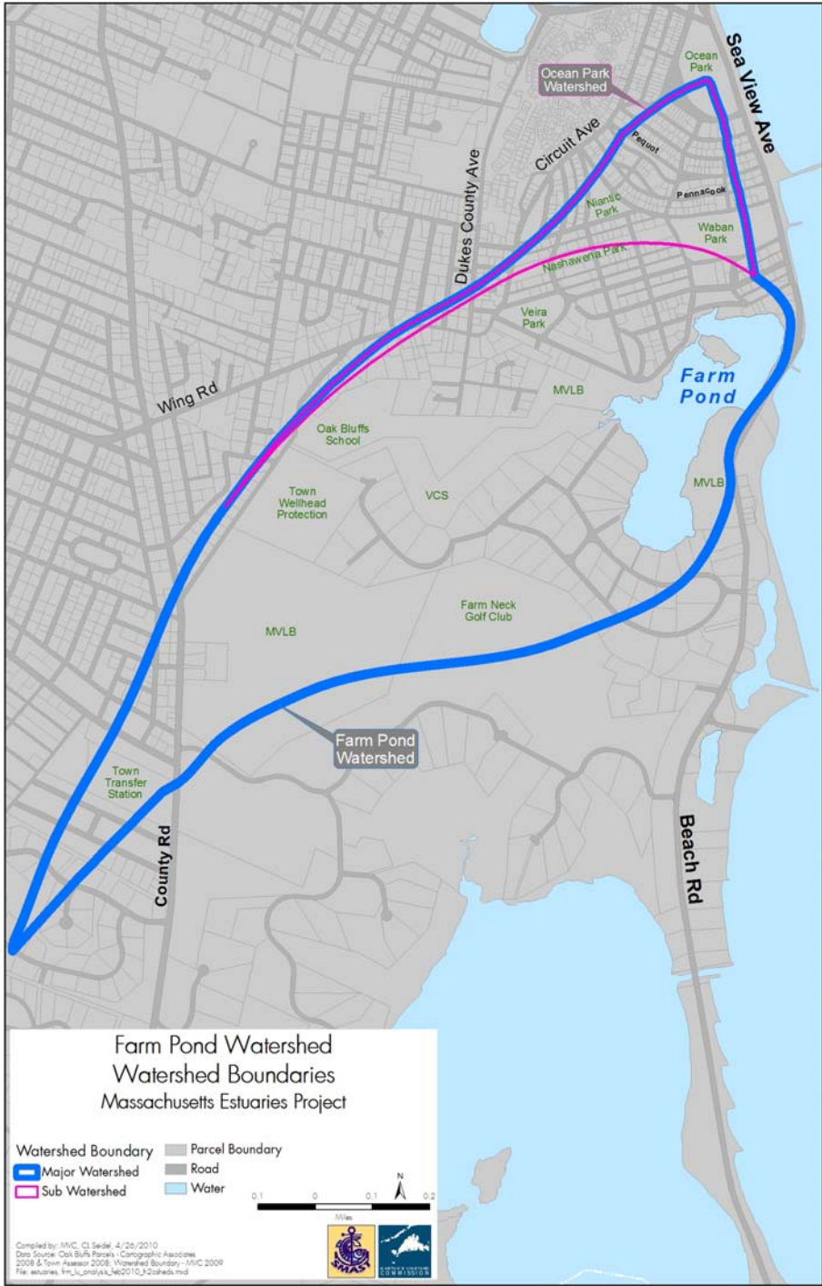
Figure III-1. Watershed and sub-watershed delineations for the Farm Pond estuary system. Sub-watersheds to embayments are based upon watershed features, such as ponds or rivers, and functional estuarine sub-units in the water quality model (see section VI).
