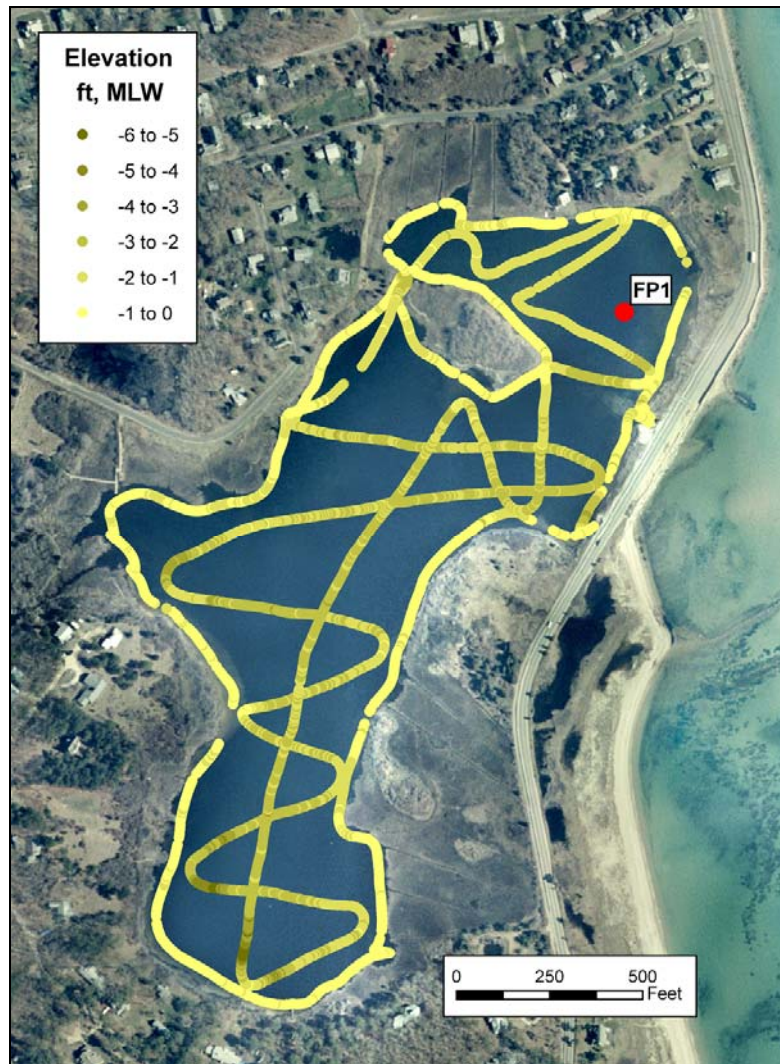
Figure V-4. Transects from the October 2005 bathymetry survey of Farm Pond. Yellow markers show the locations of the three tide recorders deployed for this study.
