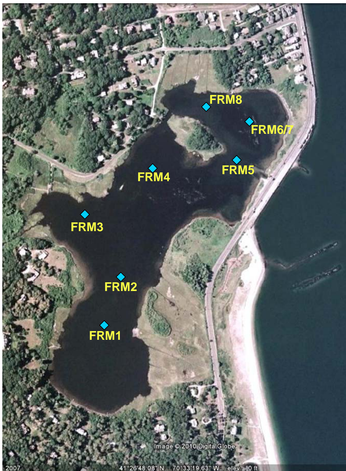
Figure IV-6. Farm Pond System locations (blue diamonds) of sediment sample collection for determination of nitrogen regeneration rates. Numbers are for reference in Table IV-3.
