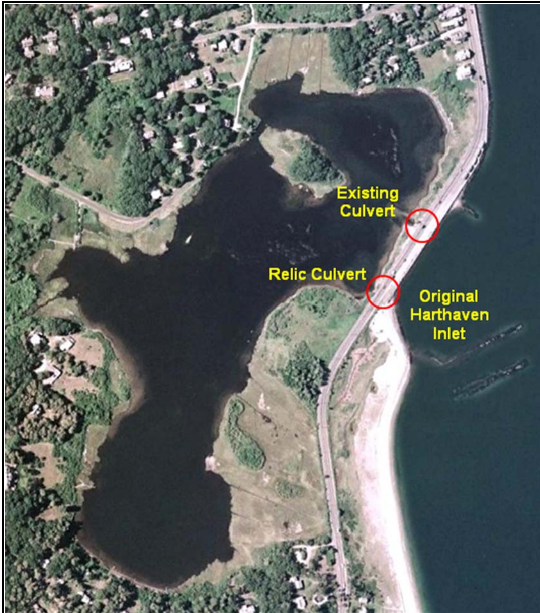
Figure I-2. Study region for the Massachusetts Estuaries Project analysis of the Farm Pond Embayment System. Tidal waters enter the Pond from Vineyard Sound through a n existing culvert passing through the barrier beach at Beach Road, and the temporarily-opened relic culvert (October 2009) which soon after being opened was clogged by a storm and abandoned. At one time Harthaven Harbor ran from the jetties (remnants seen offshore in photo) to the southern basin of the present Harbor (Figure I-1). Freshwater enters from the watershed primarily through direct groundwater discharge as there are no significant surface water inflows to this system. The island (Woody Island) was "created" by putting a channel through the base of what was a peninsula. Farm Pond is a highly man-altered system behind a very dynamic barrier beach.
