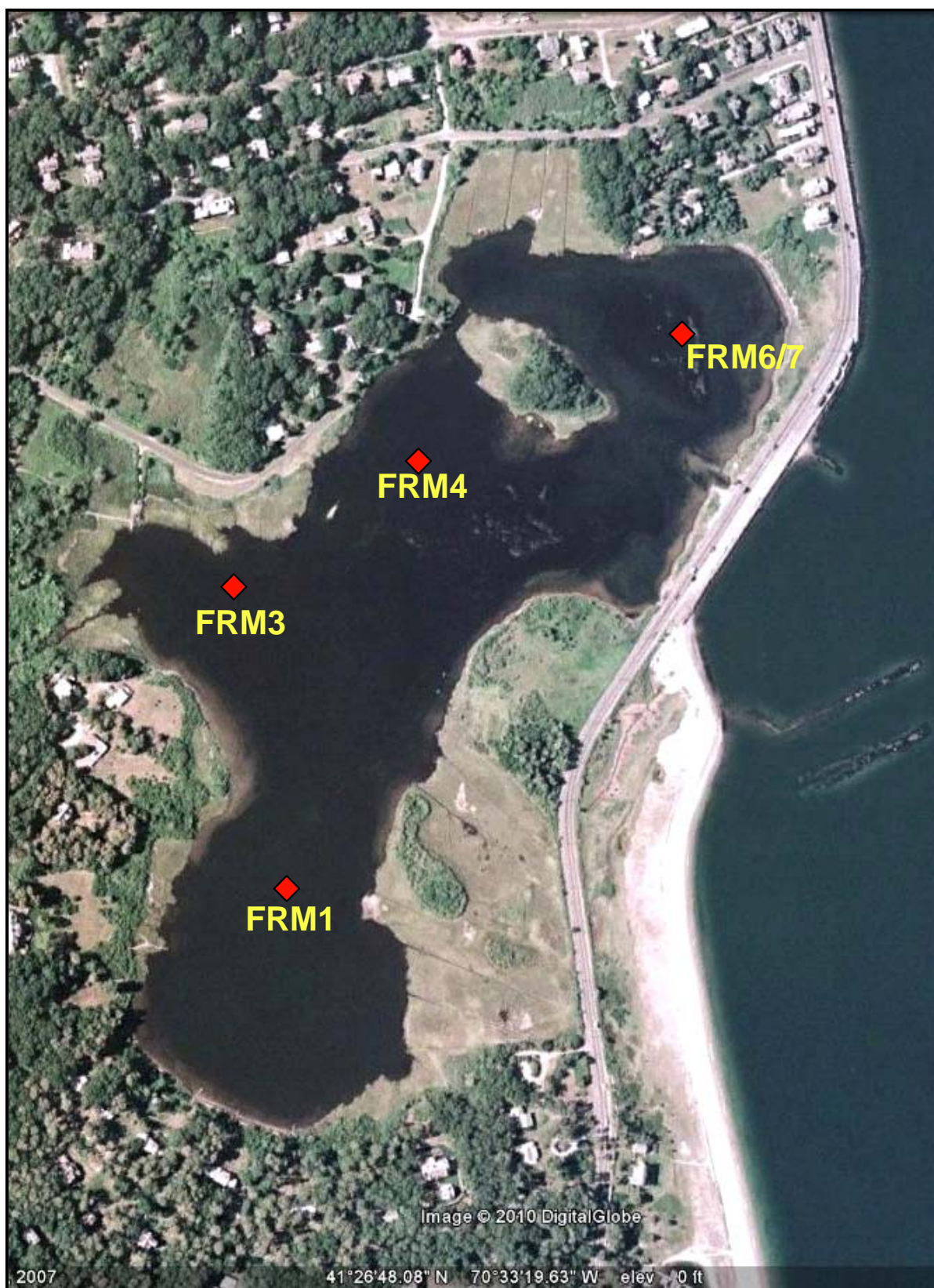
Figure VII-8. Aerial photograph of the Farm Pond system showing location of benthic infaunal sampling stations (red symbol).
