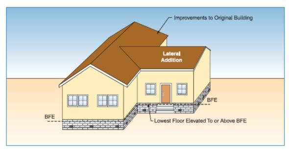
Figure 6-4. Lateral addition to a pre-FIRM building in an A zone – the proposed work includes an addition and work on the original building, including structural modification of the common wall or roof. The proposed work was determined to be a substantial improvement. The addition complies with all requirements and the building is brought into compliance by elevating it on a compliant foundation.
