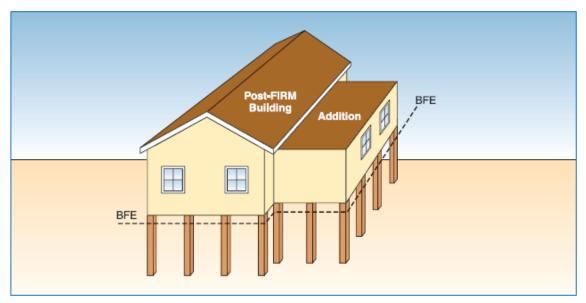
Figure 6-8. Lateral addition to a post-FIRM building in any flood zone (map revision has not changed the effective BFE). All improvements or repairs to a post-FIRM building must comply with the NFIP requirements regardless of the value of that work, and the work shall not compromise any of the NFIP requirements that the building was required to meet when it was initially built.
