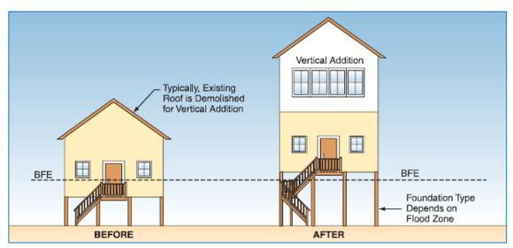
Figure 6-10. Vertical addition to a pre-FIRM residential building (in any zone) – the proposed work is a new <u>upper</u> story that involves structural modification. The work is a substantial improvement. The building is elevated to or above the BFE on a compliant foundation.
