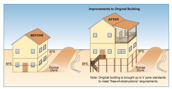
Figure 6-5. Lateral addition to a residential building in a V zone – the proposed work includes work on the original building. The lateral addition and improvements constitute substantial improvement. Both the addition and the original building are brought into compliance by elevating to or above the BFE on an open foundation.
