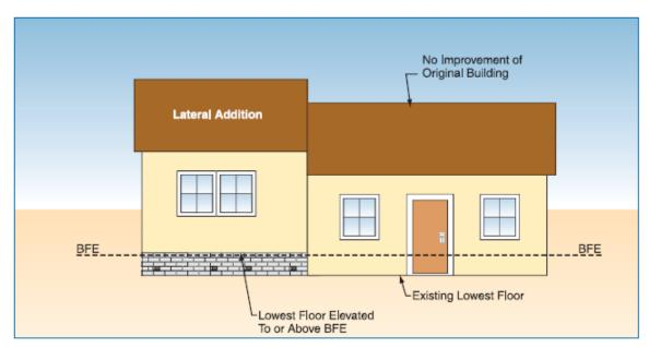
Figure 6-3. Lateral addition to a pre-FIRM building in an A zone – the proposed work is only the addition (no work was performed on the original building and no structural modification was made to the common wall or roof). The addition constitutes a substantial improvement and it complies with all NFIP requirements.
