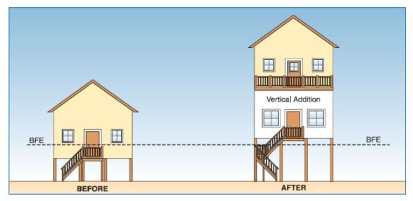
Figure 6-11. Vertical addition to a pre-FIRM residential building (in any zone) – the proposed work is a new <u>lower</u> story that involves structural modification. The work constitutes a substantial improvement. The building and the new lower story are elevated on a compliant foundation.
