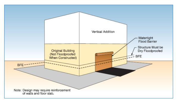
Figure 6-12. Vertical addition to a pre-FIRM, non-residential building in an A zone. The work constitutes a substantial improvement. The building is brought into compliance by retrofit dry-floodproofing measures (certification of design by registered design professional is required). Non-residential buildings can also be brought into compliance by elevation (not shown).
