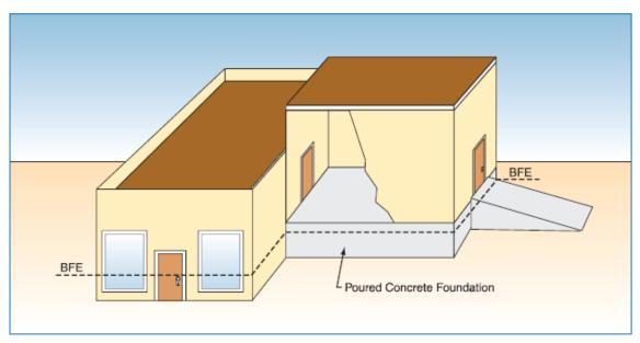
Figure 6-7. Lateral addition to a non-residential building in an A zone – the proposed work is only the addition (no work on the existing building and no structural modification of the common wall or roof). The work constitutes substantial improvement. The addition is elevated to or above the BFE (an alternative would be to dry floodproof only the addition, including the common wall).
