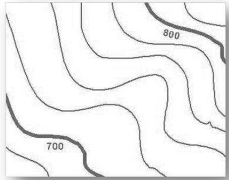
**Figure 2.13: Example of contour lines and contour interval**
