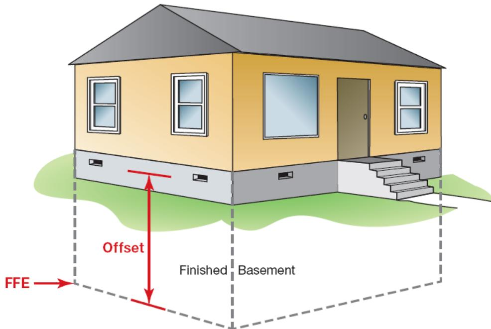
**Figure 2.8: FFE and DDF offset for finished basement**
