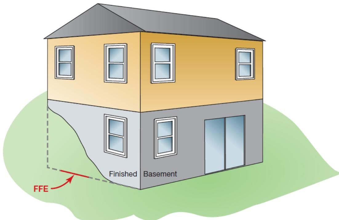
**Figure 2.9: FFE for a finished walkout basement**
