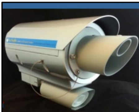
Figure 2.4: Existing non-contact road surface condition sensor at existing highway instrumentation stations - IceSight-2020E
