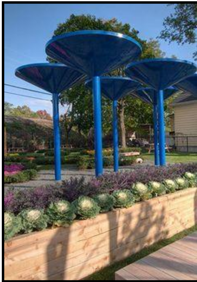
Figure 20 Rainwater harvesters and decorative stormwater planters. These cisterns contain spigots at the base to allow for re-use of the water.
