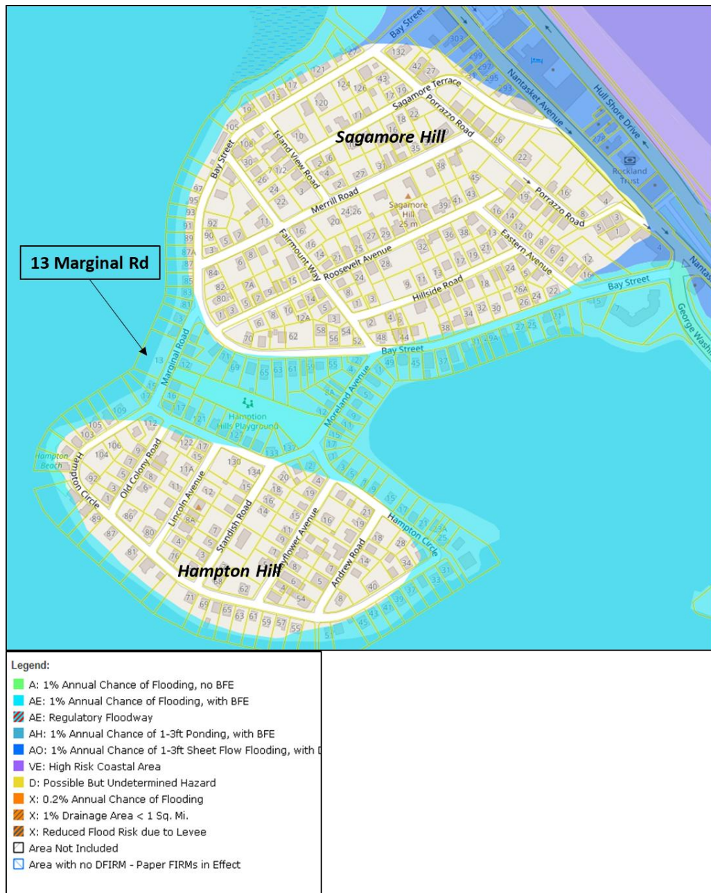
Figure 5. FEMA flood map data provided by ResilientMA.org. The proposed project site, 13 Marginal Road, is located within the AE zone, indicating a 1% annual chance of flooding. When the project area is flooded, Hampton Hill becomes isolated from the main Hull peninsula.
