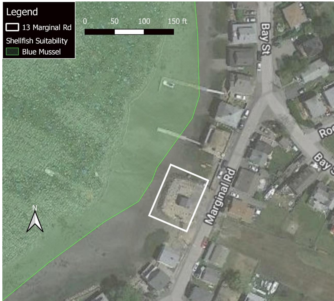
Figure 7. Approximately 25 feet seaward of the toe of the revetment is a shellfish suitability area for blue mussels shown with green hatching.
