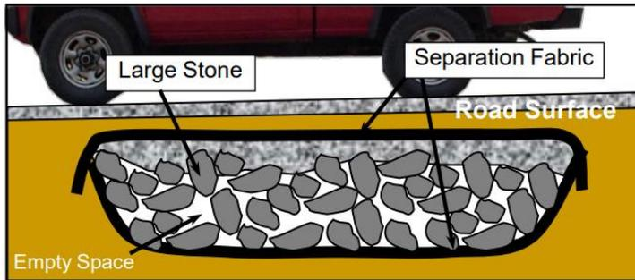
SIDE VIEW SCHEMATIC OF A FRENCH MATTRESS (SOURCE: PENN STATE CENTER FOR DIRT AND GRAVEL ROAD STUDIES)
