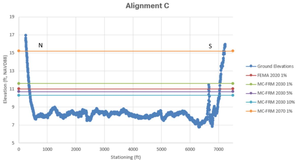
**Figure 4-5: Alignment C Elevations**
