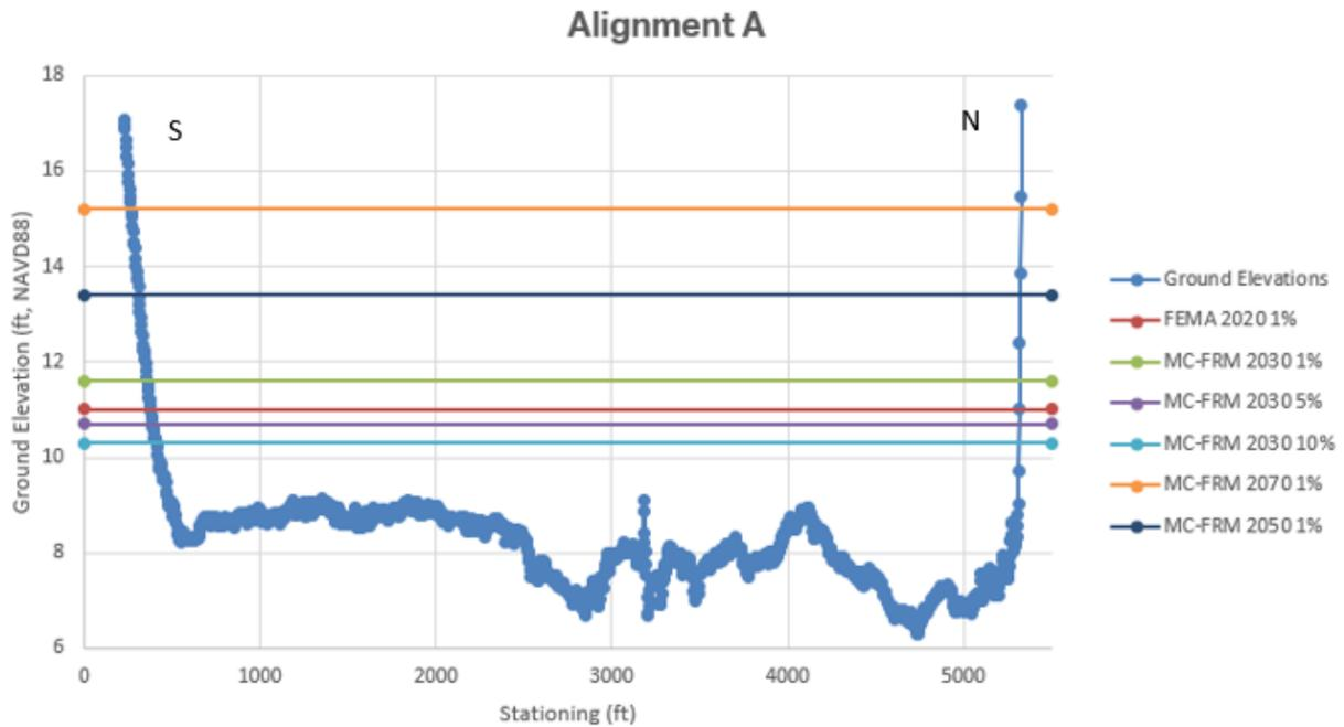
**Figure 4-3: Alignment A Elevations**
